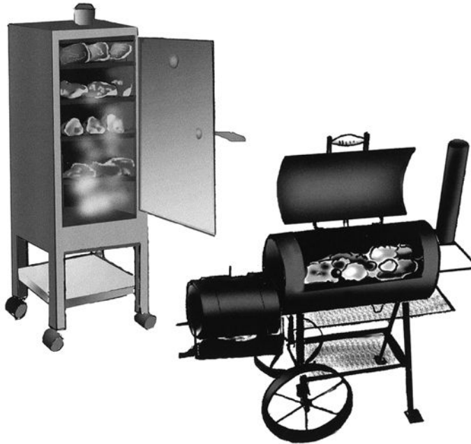
Figure 2-1: On a vertical charcoal smoker (left), the meat cooks far above the heat. An offset horizontal smoker separates the fire and the cooking surface.
