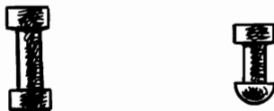
Figure 27. The spool pin is at left, and the mushroom pin is at right.
