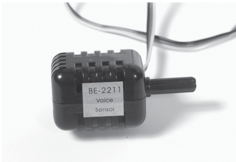
Figure 72-1 This voice sensor in the JoinMax RoboEXP Educational Kit can be used for controlling your robot via sound/noise.
