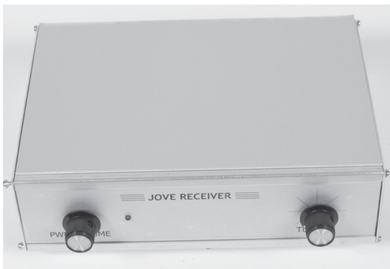
Figure 30-43 Test fit the chassis top panel.
