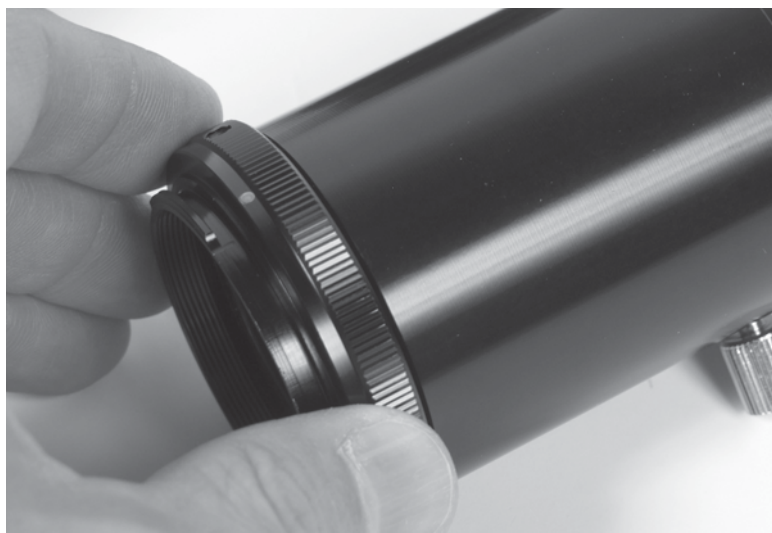
Figure 61-4 Add the T-Mount to the camera adapter.
