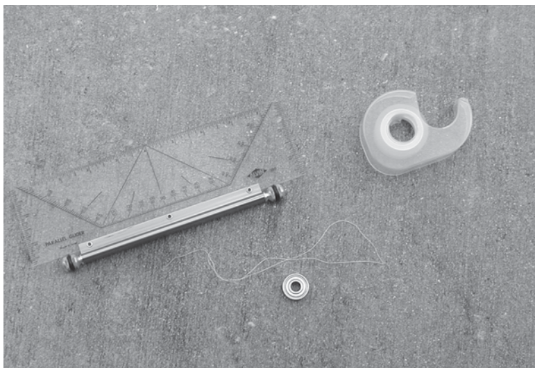
Figure 3-2 A simple protractor, a weight, some thread, and a little tape can build a device for measuring the angle used in calculating altitude.
