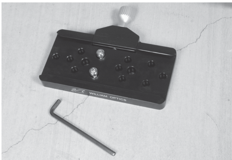
Figure 58-31 Prepare the Vixen-style dovetail telescope mount plate.
