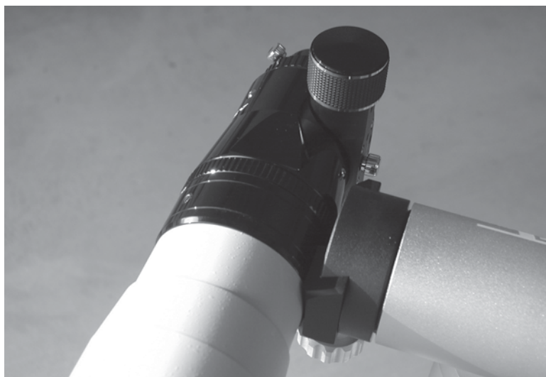
Figure 58-42 Slip the AT66ED into the dovetail mount of the Eazy Touch ALT-AZ mount.
