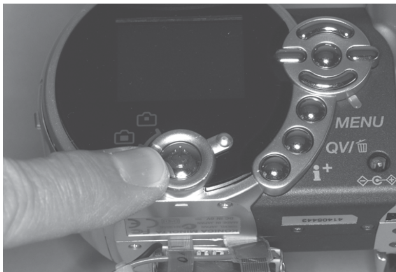
Figure 64-45 Turn on the external battery pack, and then turn on the camera.
