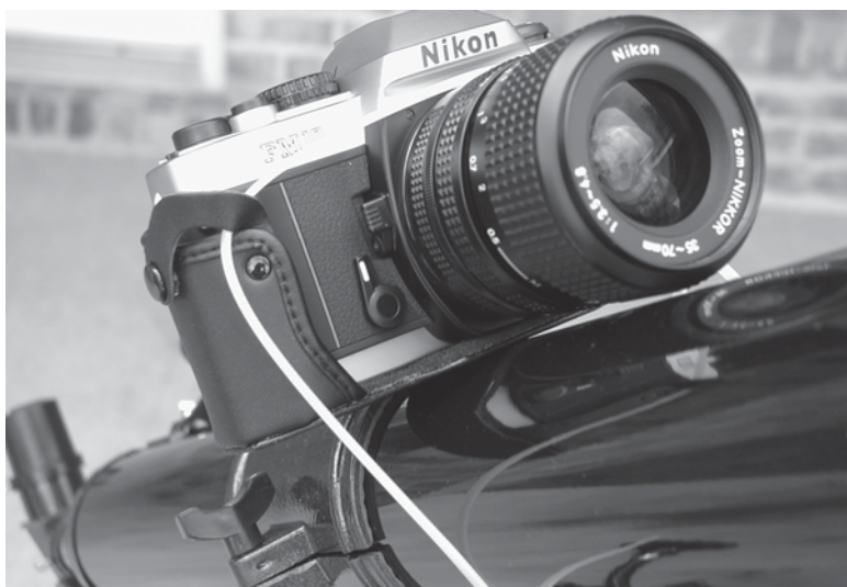
Figure 63-4 Loop a cable tie through your camera's case for providing a stable attachment platform.
