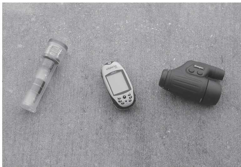
Figure 62-1 The three essential devices for a star party field kit: Great Red Spot Junior Red LED Shake Flashlight (left), Magellan eXplorist 210 (center), and Night Owl Optics Night Vision Scope (right).
