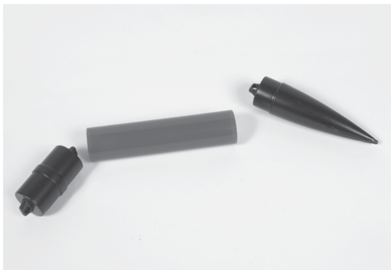
Figure 20-1 Only two extra parts are needed for building a payload-lifting model rocket—a connector or joiner tube and a payload tube.
