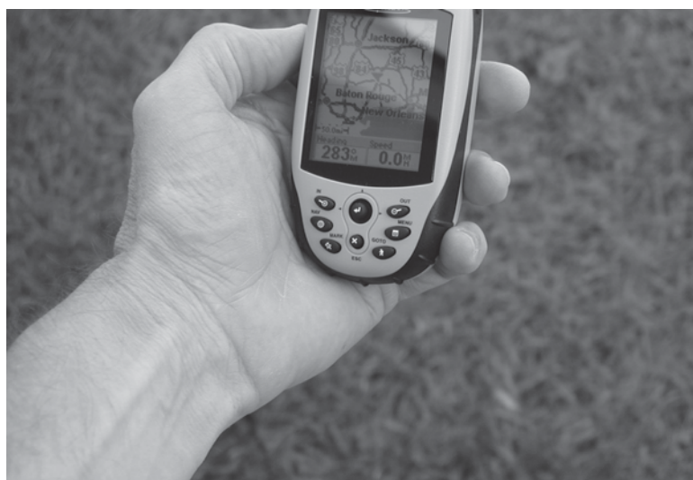
Figure 9-8 You can zoom in on your present location with the Magnify button.
