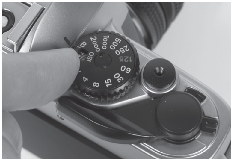
Figure 60-8 You will be primarily using the B or Bulb shutter-speed setting for astrophotography.
