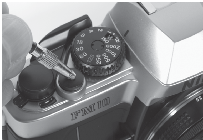
Figure 60-11 Thread the cable release into the shutter release button.
