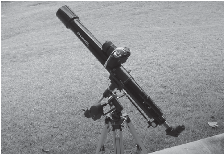
Figure 63-6 When mounting your camera on your telescope for deep space photography, make sure the camera's field-of-view clears all obstructions on the telescope. This check is best performed during the daylight, before you begin to take your photographs.
