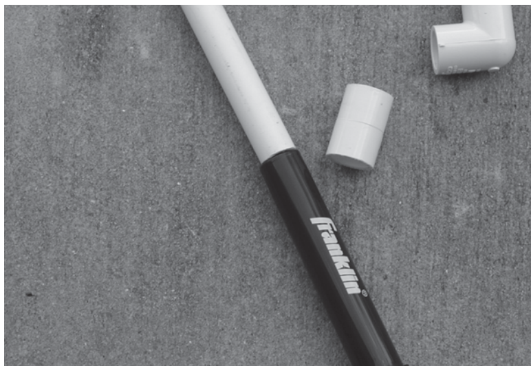
Figure 14-2 The pump is connected to the “launch pad” via PVC tubing.
