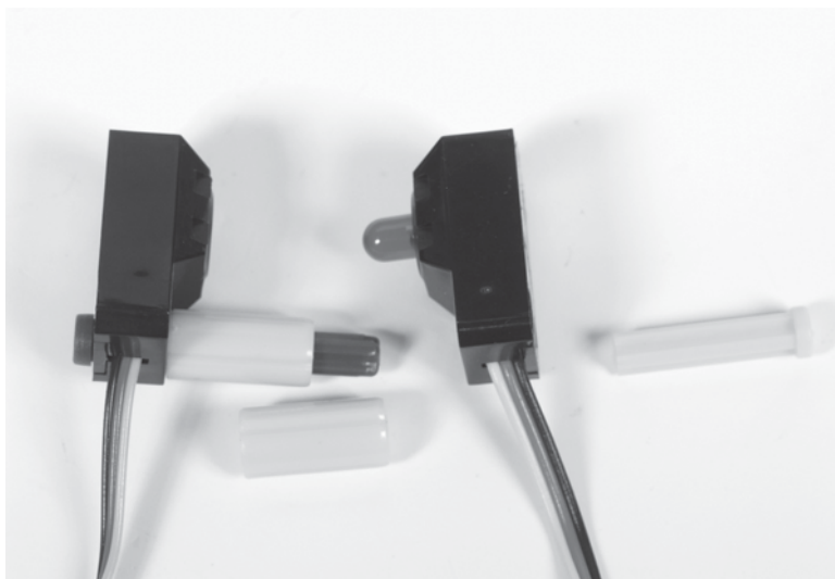
Figure 71-3 A crude light-wave communication system can be built from the photoresistor light sensor and the LED module.
