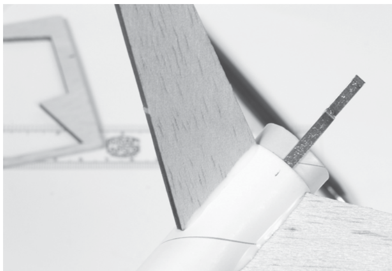
Figure 15-26 Add glue fillets to both sides of each fin. This action reinforces each fin, as well as streamlines the air flow along the rocket's body.
