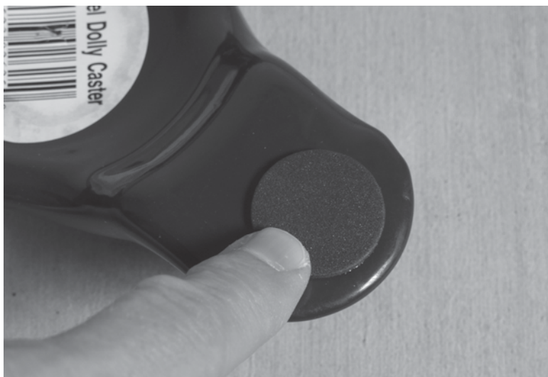
Figure 54-27 Just make sure your dolly has friction pads for keeping your dolly underneath your Dob.
