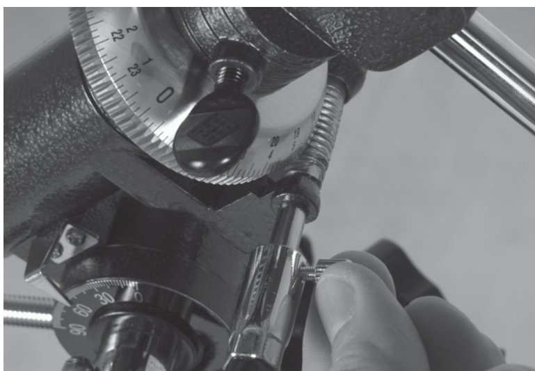
Figure 53-18 Attach the long flexible cable to the right ascension worm drive.
