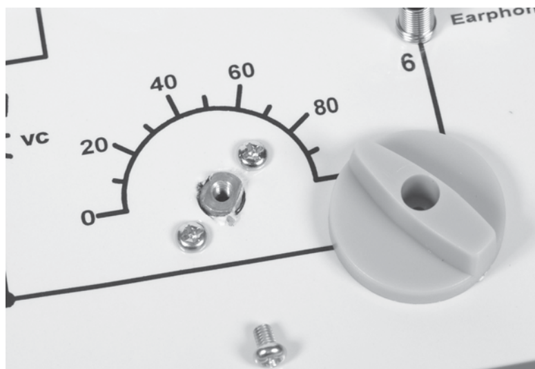
Figure 26-12 Two screws hold the tuning capacitor.
