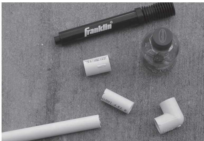
Figure 14-1 You can build a water-powered rocket from an old water bottle, some PVC plumbing tubing, a rubber seal, fasteners, and a bicycle pump.
