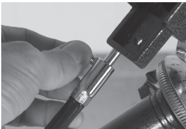
Figure 53-17 Attach the short flexible cable to the declination worm drive.
