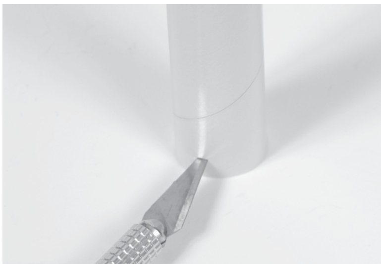
Figure 15-8 Cut a small slit in the motor mount.
