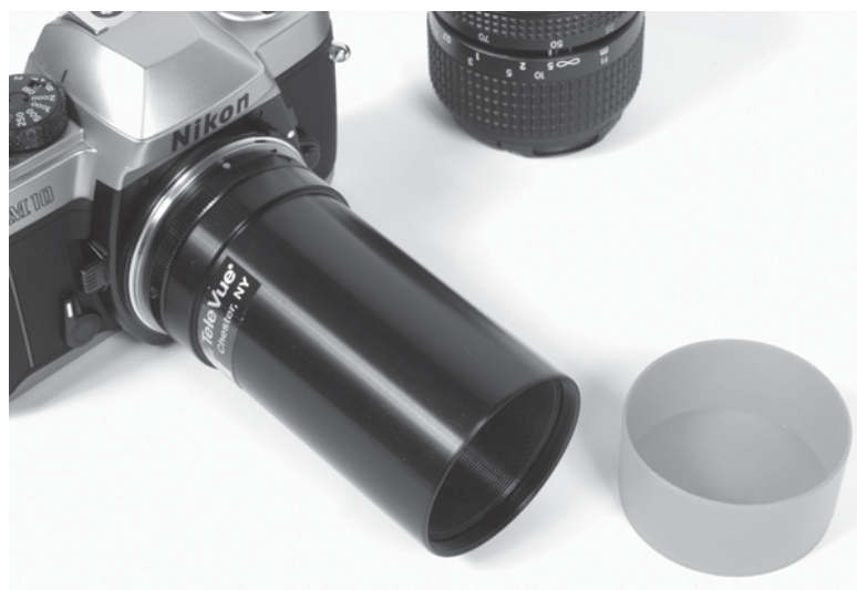
Figure 61-9 Mount the adapter on the camera and use the camera/adapter in lieu of an eyepiece.
