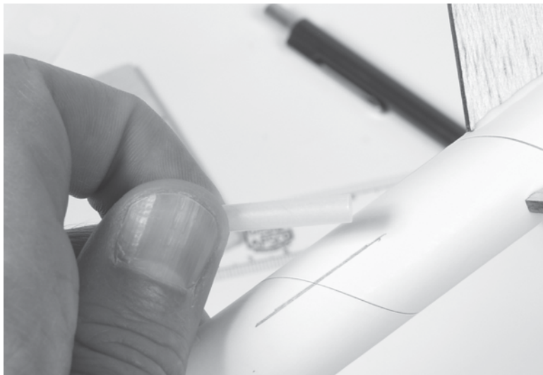
Figure 15–27 Attach the launch lug to the main rocket body tube.
