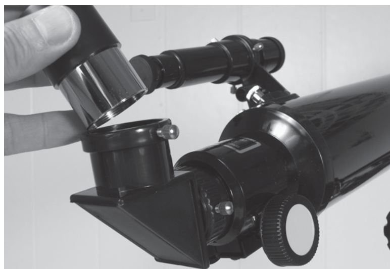
Figure 52-28 Slip an eyepiece into the diagonal.
