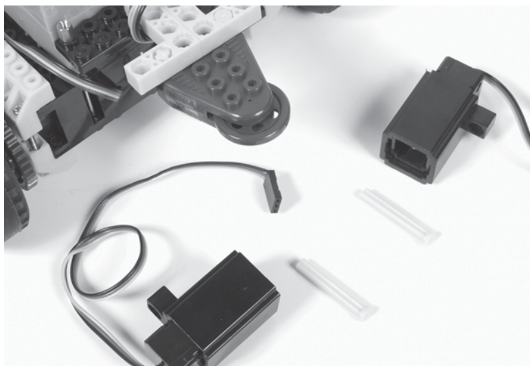
Figure 71-1 Several nifty light sensors are included with the 0600 JoinMax robot kit. These gray sensors can be used for following a line or checking for edges and cliffs. Yikes!
