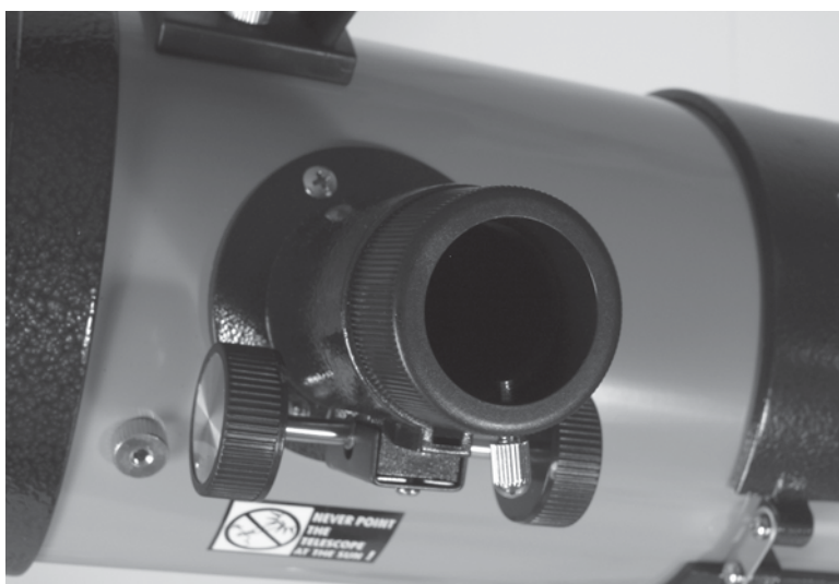
Figure 53-28 No diagonals are needed with a reflector telescope. Eyepieces are inserted directly into the focusing tube.
