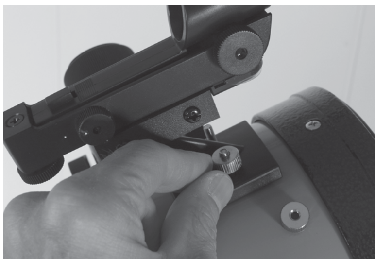
Figure 57-9 Secure your finder scope to your telescope tube.
