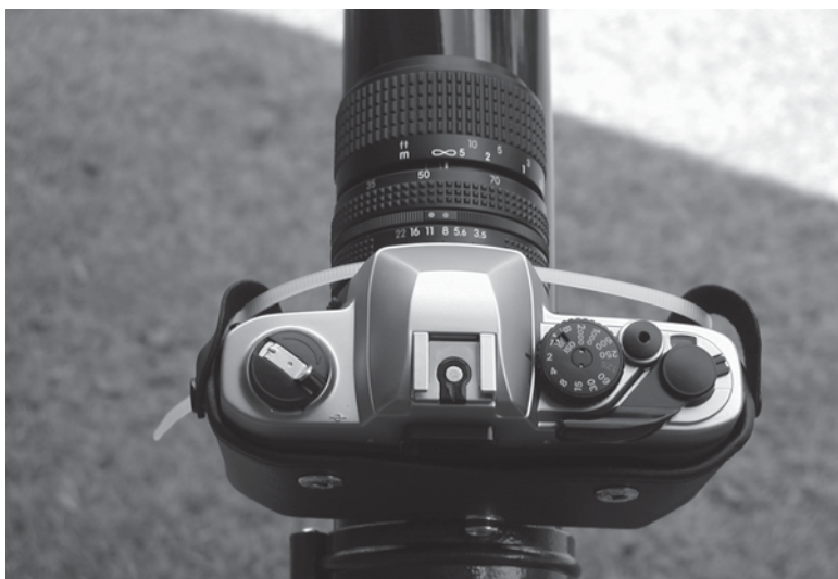
Figure 63-7 Align the camera perfectly with the telescope tube. Then, the telescope's motor drive can be used for tracking your deep-sky object.
