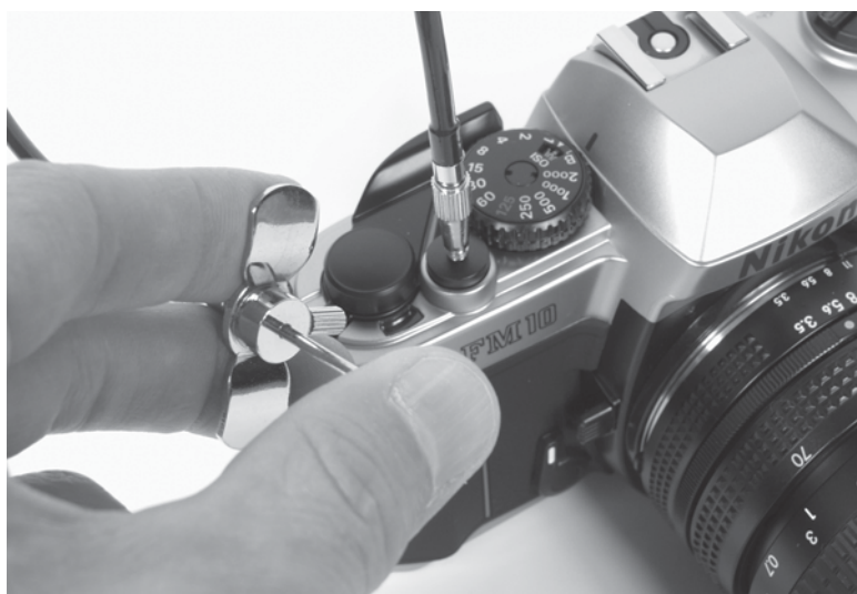
Figure 60-13 Now you can remotely trigger the camera's shutter without touching the camera.
