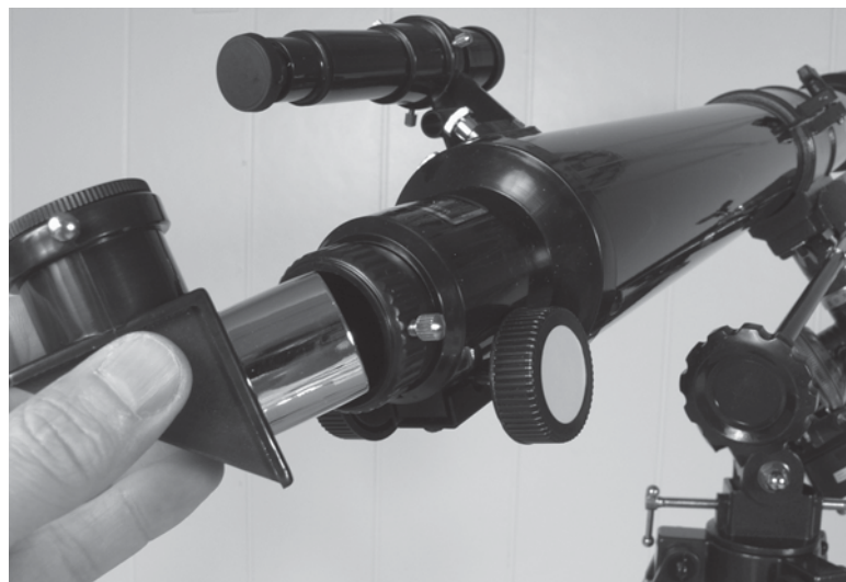
Figure 52-26 Attach the diagonal to the telescope's focusing tube.
