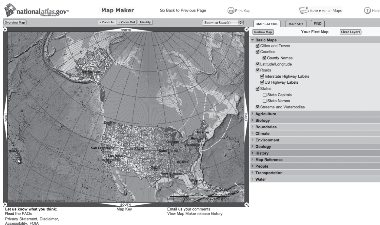
Figure 2-1 Map Maker from the National Atlas website ( nationalatlas.gov ) displays lines of magnetic variation.
