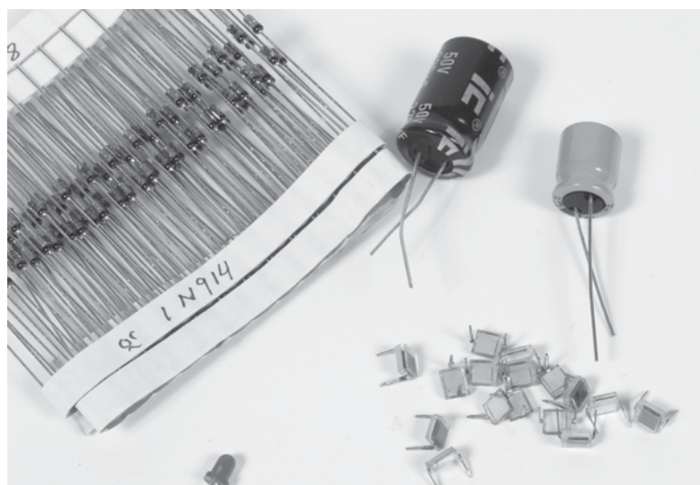
Figure 69-2 Just a handful of discrete analog components are needed for building your own solar power generator. The BPW33 photodiodes (lower right) also generate electricity when exposed to light.
