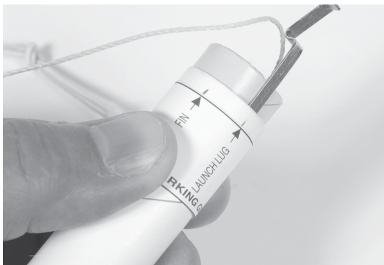
Figure 15-18 Mark the main rocket body tube for the fins and launch lug.
