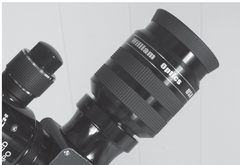
Figure 58-41 The Astro-Tech AT66ED includes a locking collar, enabling you to rotate the focuser to any desired viewing angle.
