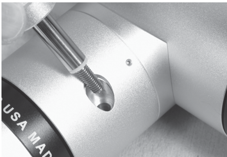
Figure 58-17 Loosely thread the azimuth adjustment set screw into place.
