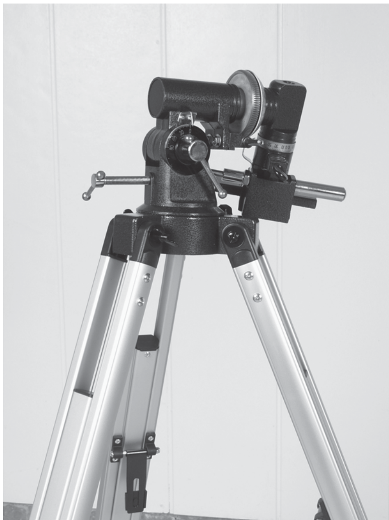
Figure 53-9 Raise the tripod and level the legs.
