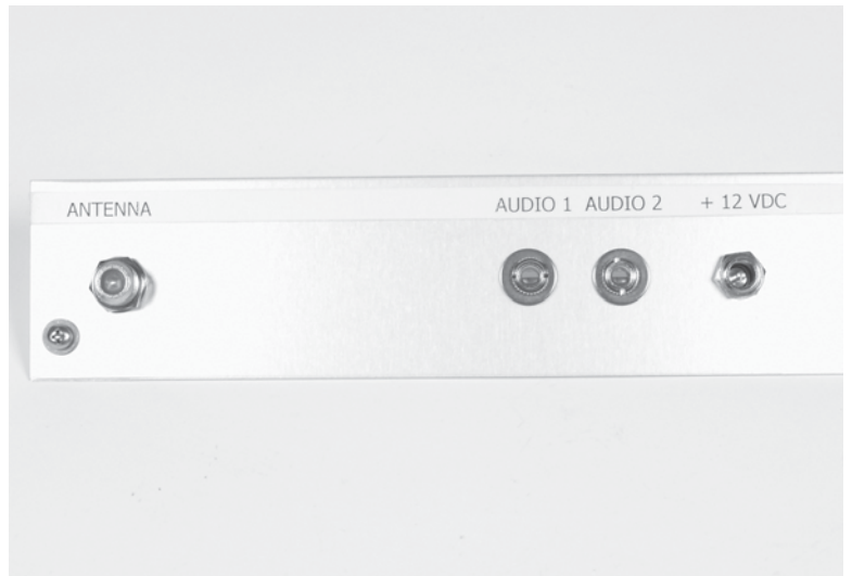
Figure 30-10 Install the jacks and lug.
