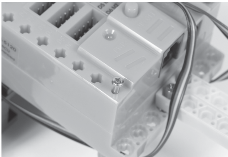
Figure 66-6 A programmable controller, the Super Robot Control Unit (RCU), controls your robot.
