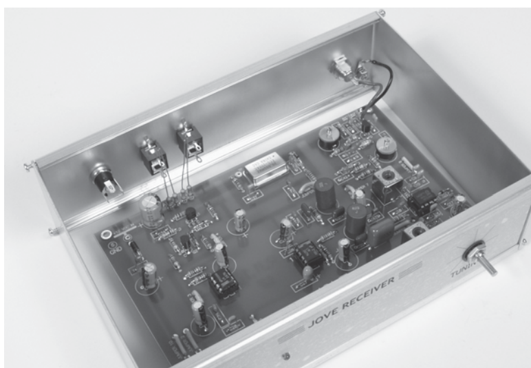
Figure 30-37 Loosely attach the chassis right side panel.
