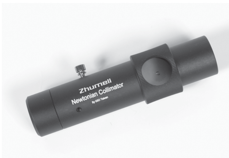
Figure 57-5 Use a collimator for aligning the mirrors in Dobsonian and Newtonian telescopes.
