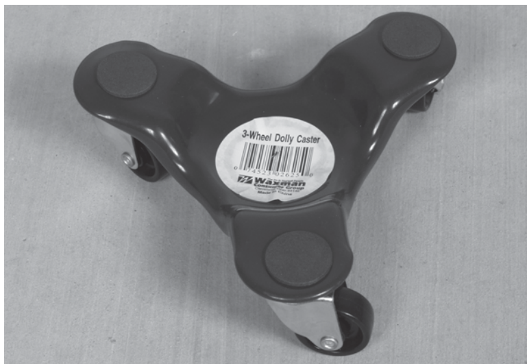
Figure 54-26 One drawback of the Dobsonian telescope is that it can be unwieldy to move. A mover's dolly is a great tool for moving your "Dob" about and can be found in most DIY hardware centers for less than $10.
