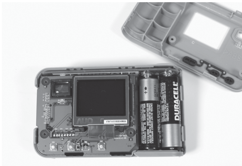
Figure 64-3 Remove the case back panel.
