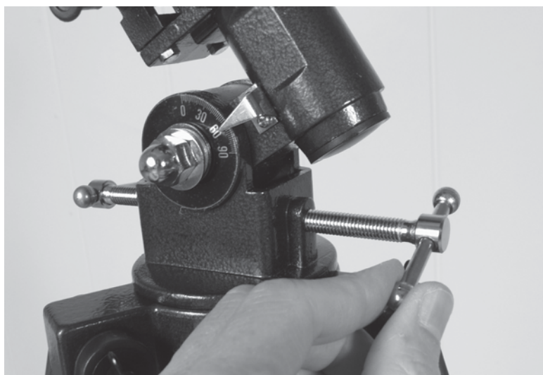
Figure 52-7 Loosen the altitude block.
