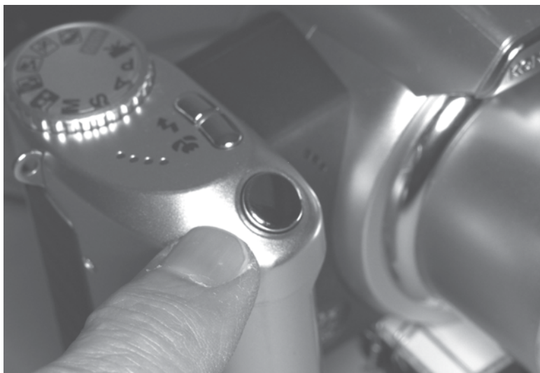
Figure 64-48 The shutter release button must either be able to capture long, extended exposures or you can use the video recording mode.
