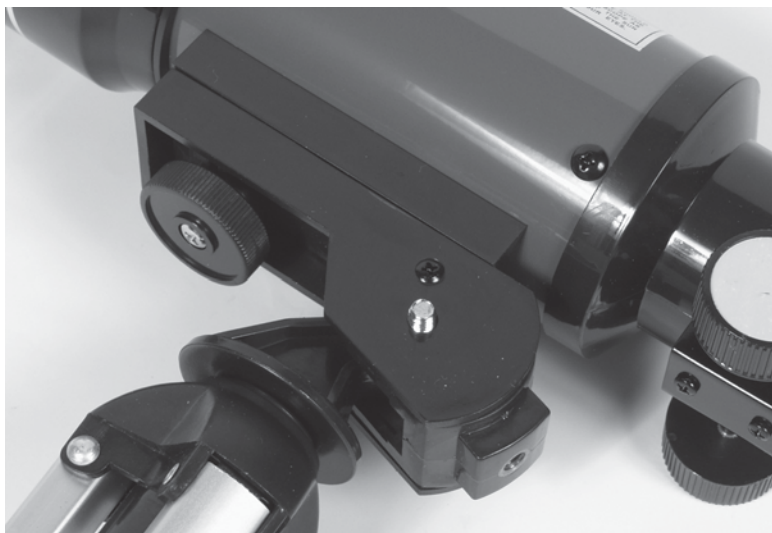
Figure 51-3 Mount the scope on its tripod.
