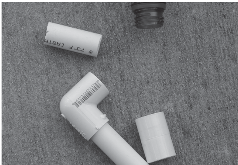
Figure 14-3 This “launch pad” holds the water-bottle rocket while air is pumped into the rocket.
