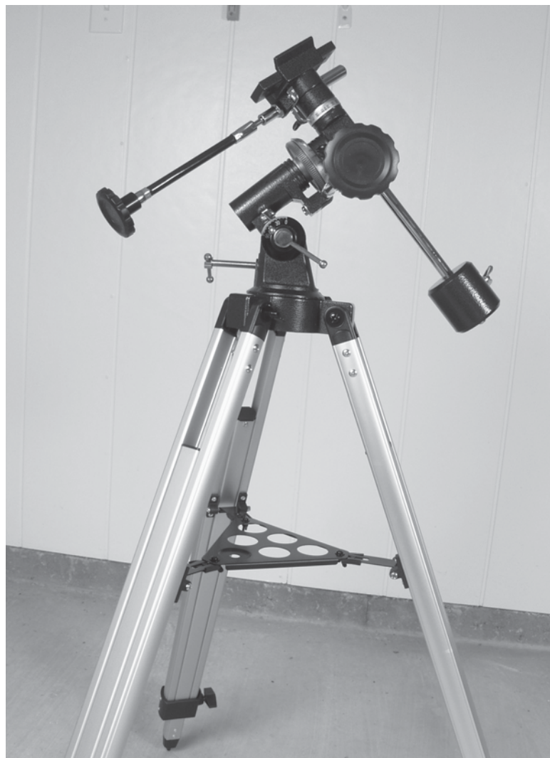
Figure 53-22 Level both the tripod and telescope mounts, and then tighten the accessory tray bolts.
