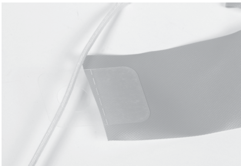
Figure 15–32 Run the shock cord through the hole in the gripper tab.
