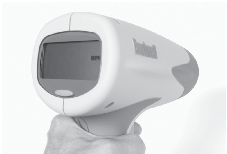
Figure 4-4 Squeezing the trigger gives you a velocity reading in miles per hour.
