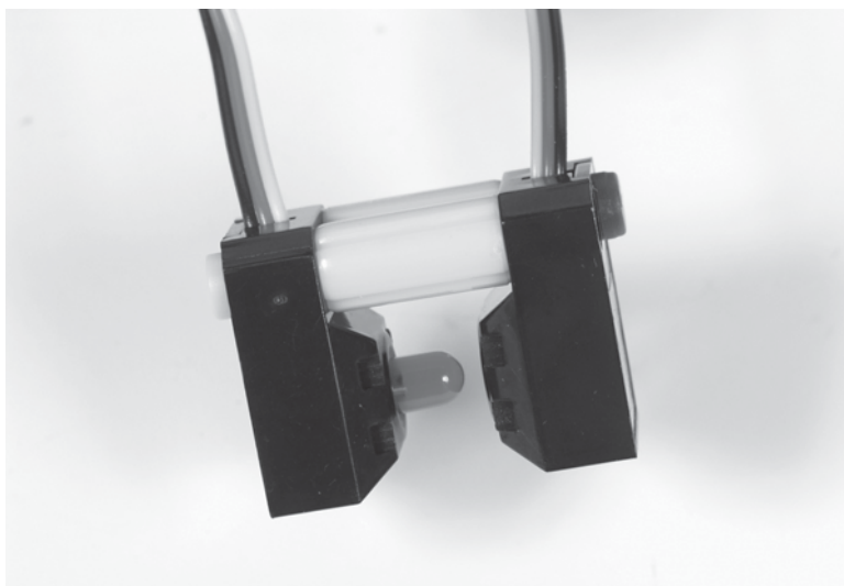
Figure 71-5 Ensure that both sensors are extremely close to each other.
