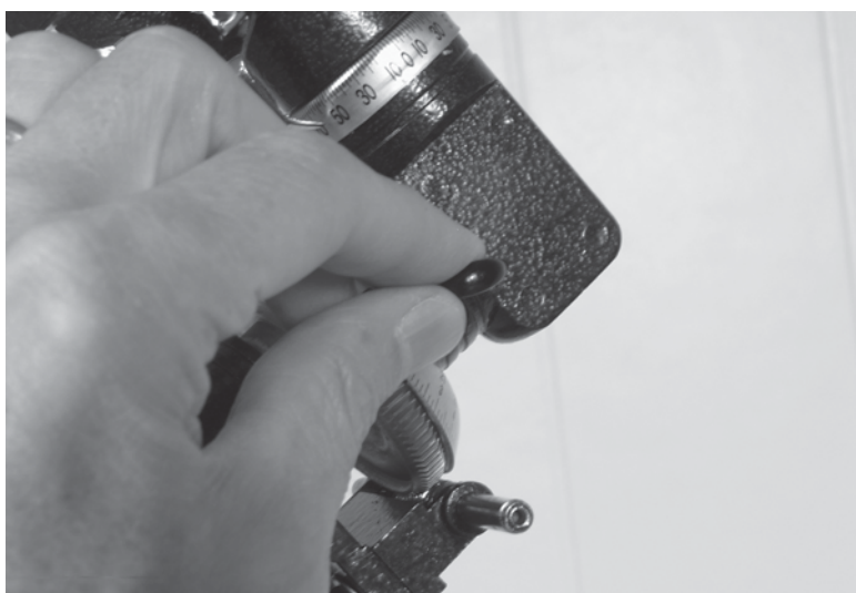
Figure 53-15 Tighten the blocking screw for the declination adjustment.
