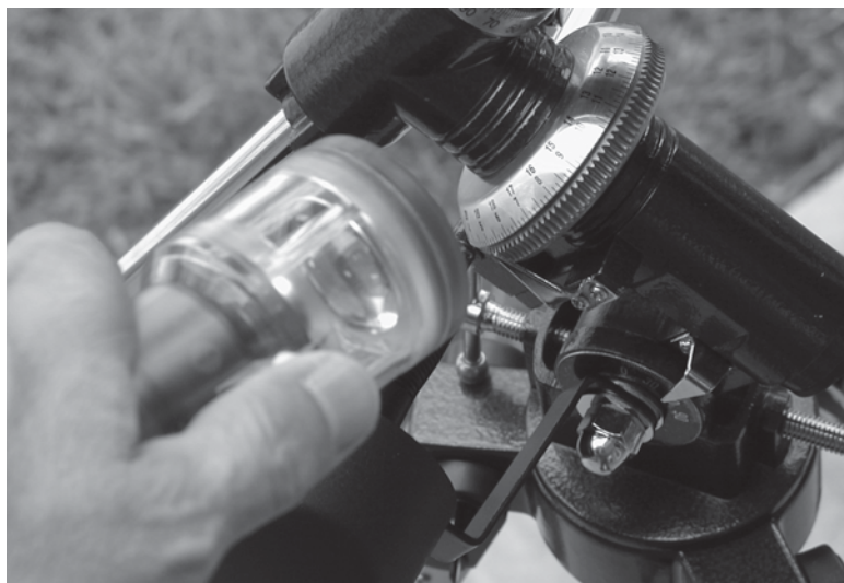
Figure 47-1 A red flashlight like the Great Red Spot Junior Red LED Shake Flashlight is ideal for reading telescope markings without compromising your night vision.
