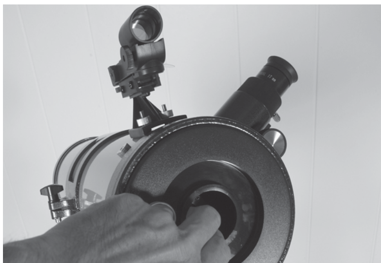
Figure 53-31 Carefully remove the lens cap. If you can't grasp the lens cap, remove the center portion for easier gripping.
