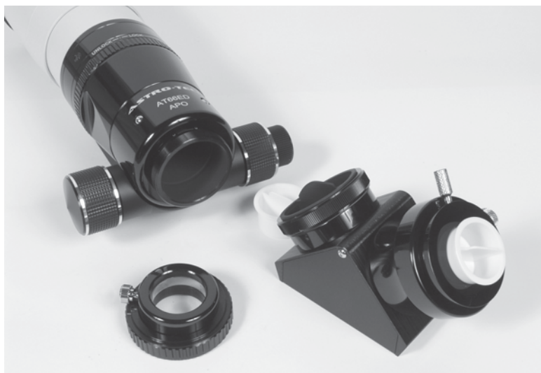
Figure 58-8 Remove the 1.25-inch eyepiece holder for adding a diagonal.
