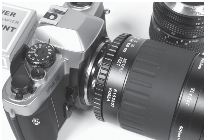
Figure 21-5 A Nikon T-Mount enables this Vivitar 500mm mirror lens to be attached to this Nikon FM10 camera.
