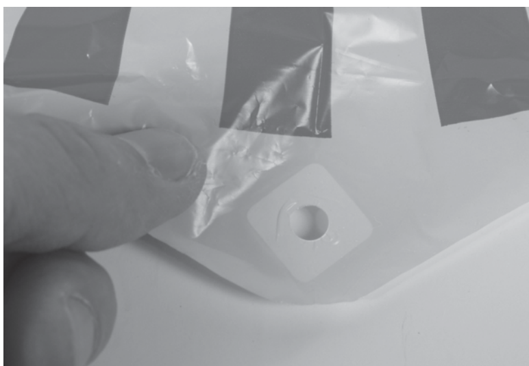
Figure 16-4 Make sure no bubbles form in the plastic parachute around each reinforcement ring.
