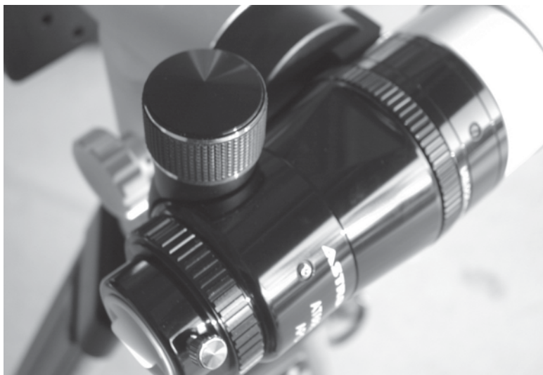
Figure 58-44 You can rotate the focuser, so the coarse focus knob is up.
