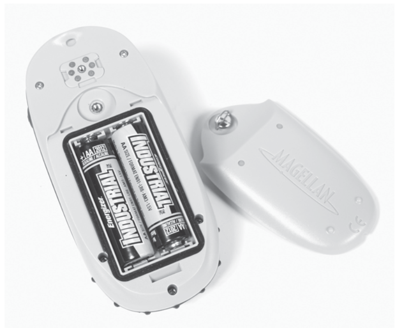
Figure 9-2 Just plop a couple of AA batteries into the eXplorist 210 and you can have the world in the palm of your hand. Well, at least you'll know where you are in the world.
