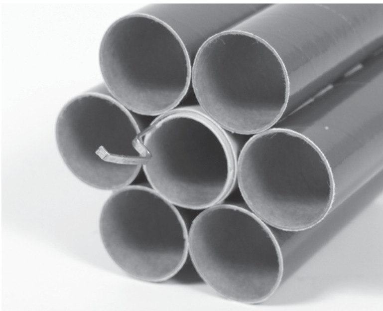
Figure 17–3 Multiengine rockets can dramatically increase the performance of your designs.
