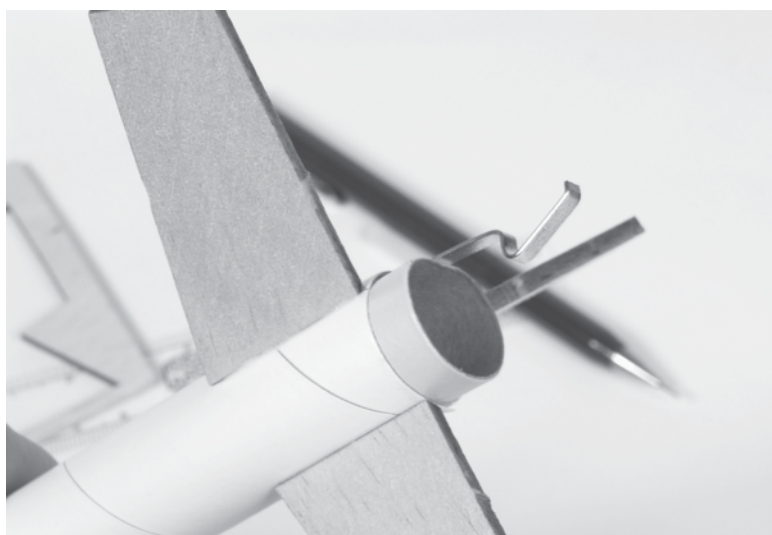
Figure 15-25 Continue to glue the remaining two fins on to the body tube.
