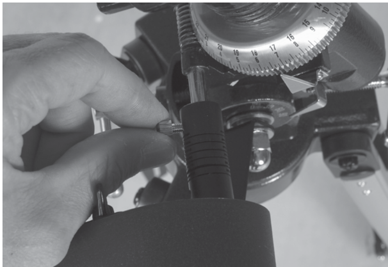
Figure 52-12 Connect the motor drive shaft to the right ascension shaft.
