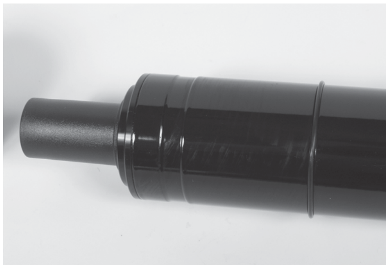
Figure 57-3 Slip the O ring into the groove on the finder scope's body tube.
