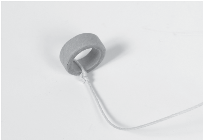
Figure 15-6 Attach the shock cord to the motor mount block.
