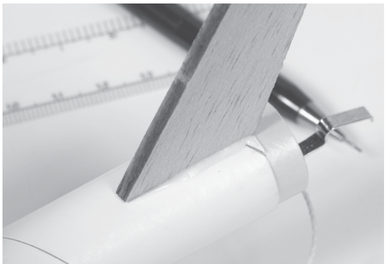
Figure 15–22 Glue the first fin to the main model rocket body tube along the previously marked line.
