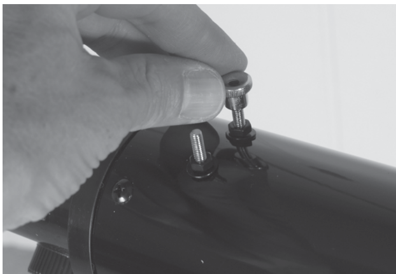
Figure 52-20 Remove the mounting nuts for the finder.
