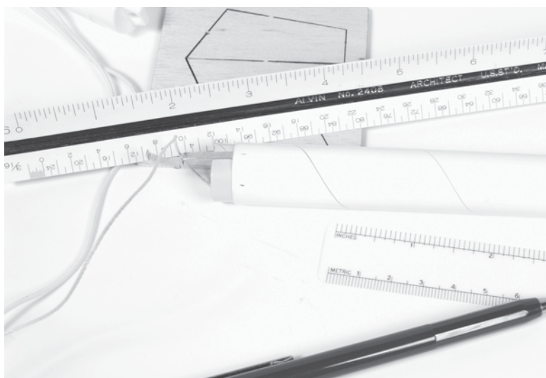
Figure 15-19 Use a grooved “architect’s scale” for extending the fin and launch lug marks along the length of the main rocket body tube.
