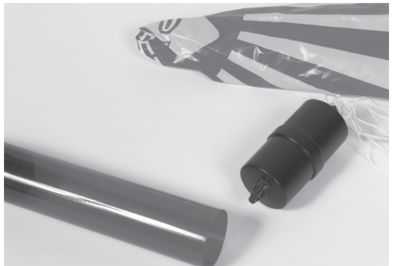
Figure 20-4 Add your payload and slip the connector tube in place on the opposite end of the payload tube.
