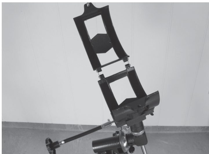
Figure 53–25 Open the saddle.
