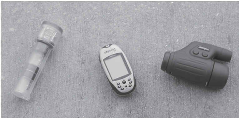
Figure 3-1 The essential star-gazing field kit (from left to right): Great Red Spot Junior Red LED Shake Flashlight, Magellan eXplorist 210, and Night Owl Optics Night Vision scope.
