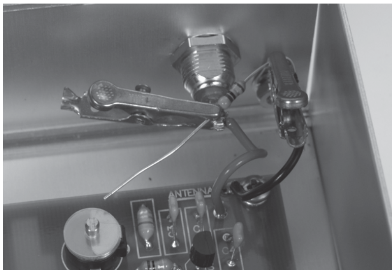
Figure 30-42 Temporarily clip a resistor across the antenna and ground lug jacks during the testing and tuning phase of the receiver assembly.
