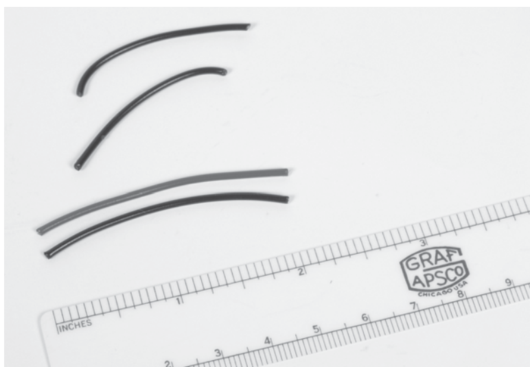
Figure 30-38 Cut wire for the power connections.
