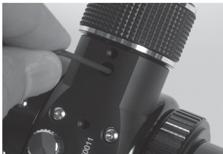
Figure 58-5 Lock the focusing knobs in place with a hex wrench.
