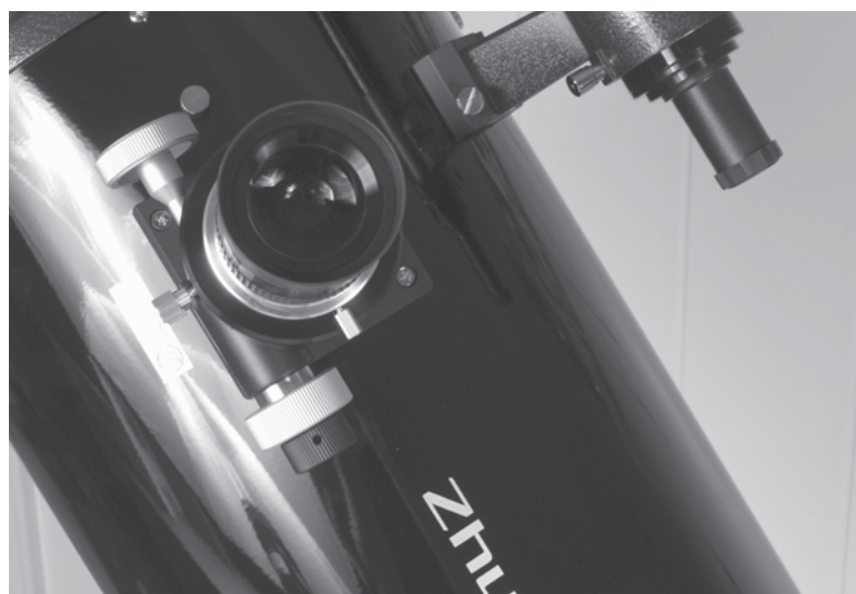
Figure 54-25 This telescope has incredible viewing power. A nice touch is the fine focus knob on the focuser.
