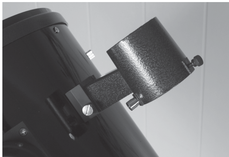
Figure 54-23 Attach the finder mount and insert the finder.
