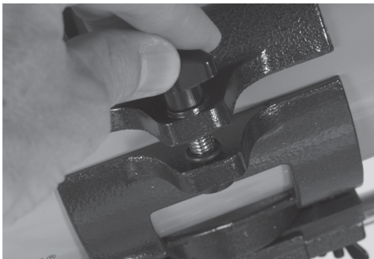
Figure 53-27 Check the balance of the telescope, and then tighten the saddle's clamp.
