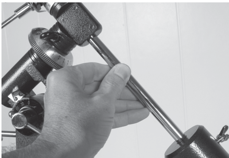
Figure 53-16 Install the counterweight.
