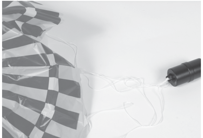
Figure 20-3 The recovery system is attached to one end of the connector or joiner tube. Unless you are a bigger evil genius than even Penelope, you should strive for a parachute recovery system.
