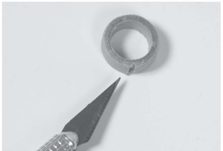
Figure 15-5 Slowly work the groove into a V-shaped slot.
