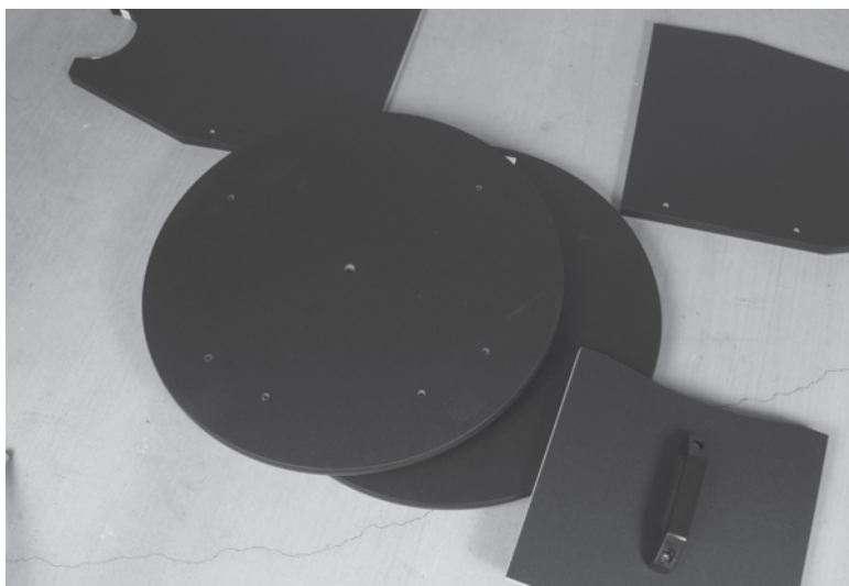
Figure 54-10 Lay the rotating plate on the mount base.
