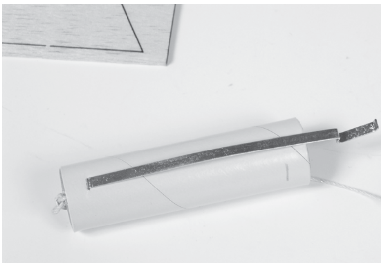
Figure 15-13 Loosely install the motor retaining clip.
