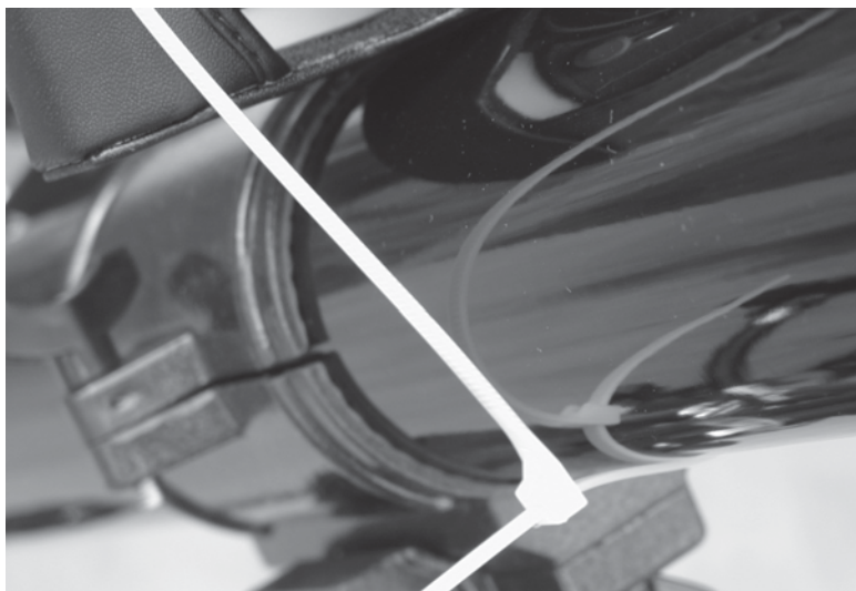
Figure 63-3 Use cable ties for mounting your camera on your telescope.
