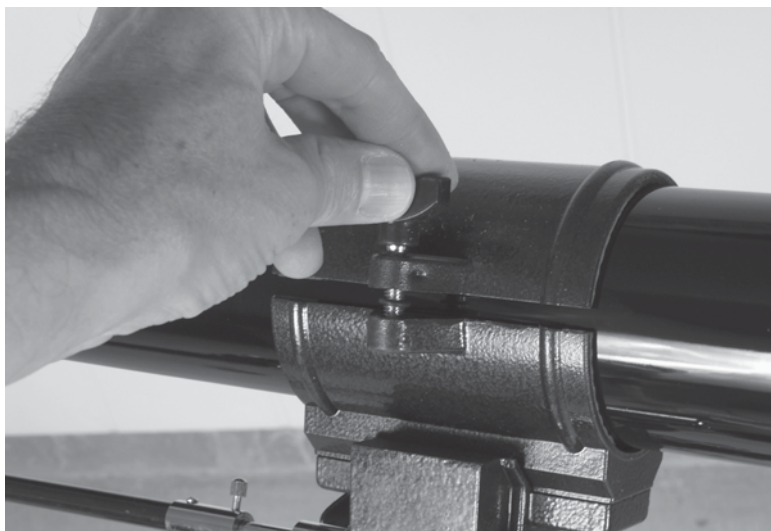
Figure 52-19 Slide the tube to a balanced point and tighten the saddle.
