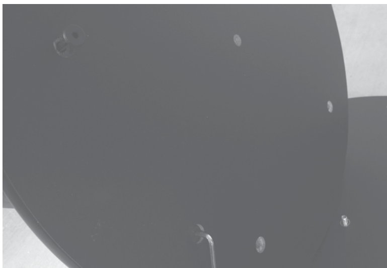
Figure 54-12 Loosely attach these screws until all sides have been assembled to the rotating plate.
