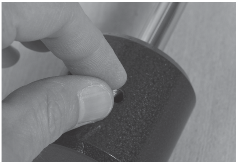
Figure 53-14 Make sure you insert the counterweight set screw in the proper orientation. If it is backward, the weight will slide loosely up and down the counterweight mounting shaft.
