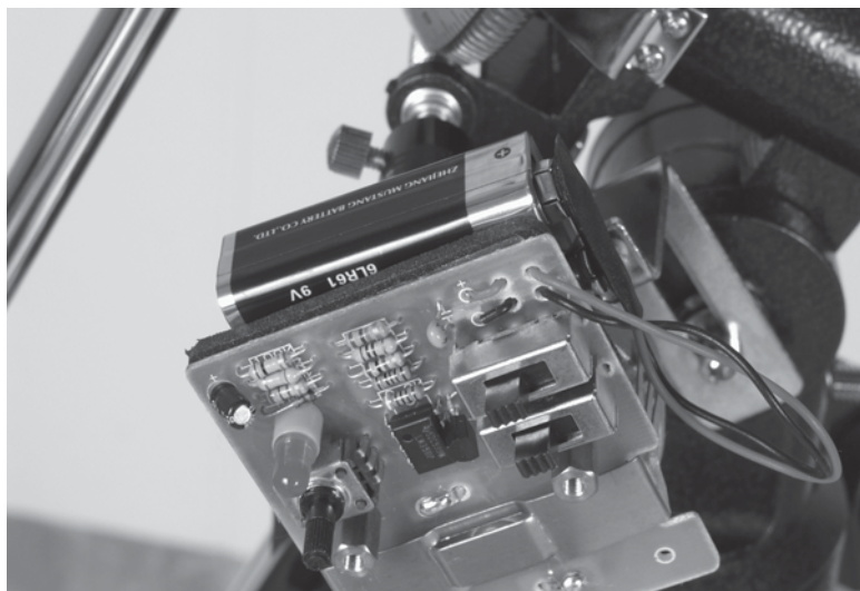
Figure 55-8 Install the battery and replace the motor drive cover.
