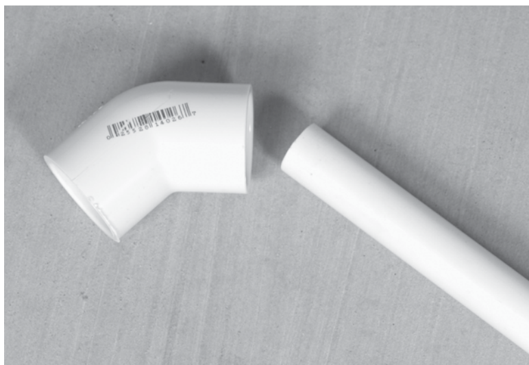
Figure 86-4 A 45° angle connector is great for adding curves to your dome. This ½-inch tubing won't fit inside the 1-inch connector without an adapter.
