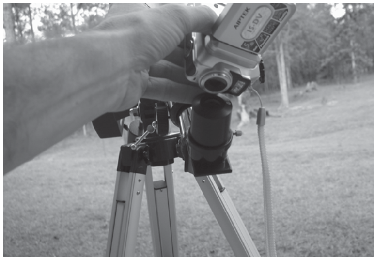
Figure 65-3 You can check your video in the field. Cover the LCD with a piece of red cellophane during viewing. This will protect your night vision.
