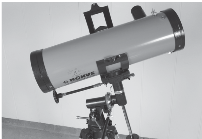
Figure 53–26 Gently lay the telescope in the saddle.
