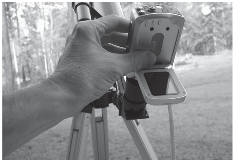
Figure 65-2 Hold your digital video camera up to the eyepiece for a painless video tour of the heavens.
