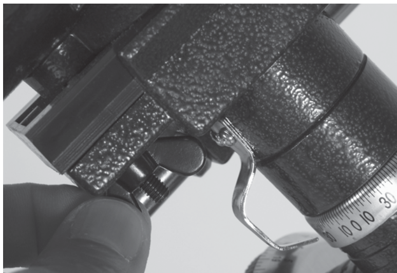
Figure 53–24 Watch the orientation of the saddle's wing nuts to ensure clearance is in all movements of operation.
