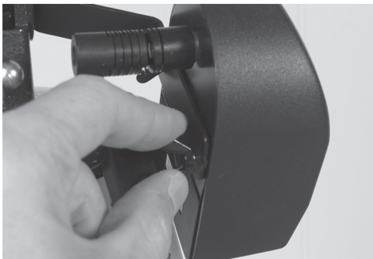
Figure 55-11 Reattach the motor drive cover and connect the motor's shaft to the RA worm drive.
