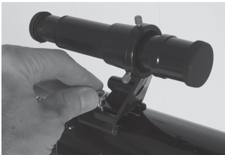
Figure 57-11 Most finder mounts have several set screws for adjusting the line of view and ensuring the scope doesn't move once you've coordinated your finder scope with your telescope.
