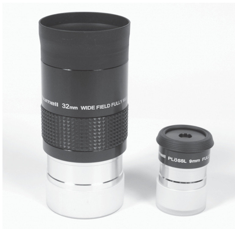
Figure 57-7 Size does make a difference: a 2-inch eyepiece (left) and a 1.25-inch eyepiece (right).
