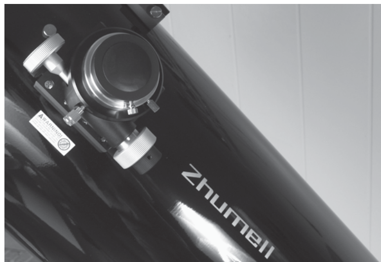
Figure 54-21 Raise and rotate the telescope tube for easy access to the focuser.
