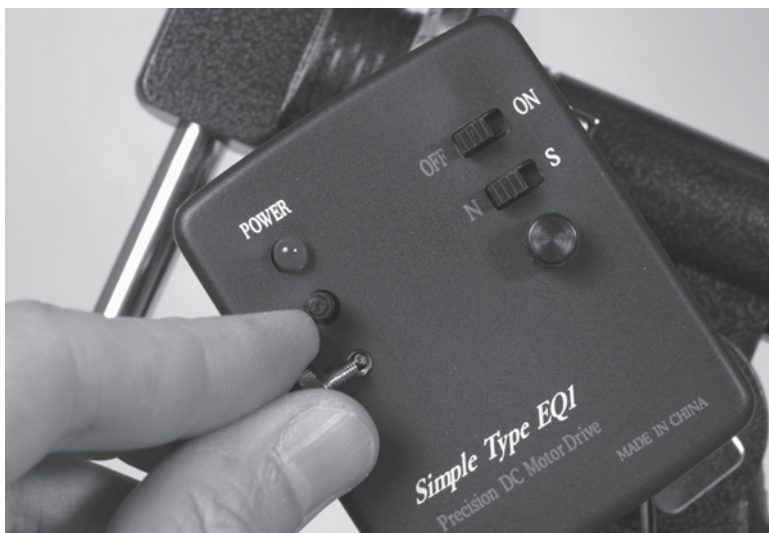
Figure 55-6 Remove the motor drive cover.
