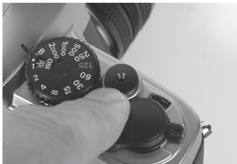
Figure 60-9 A threaded shutter release button is needed for adding a cable release.
