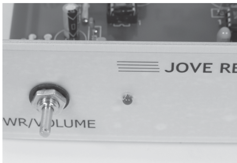
Figure 30-31 Mount the LED to the front panel.
