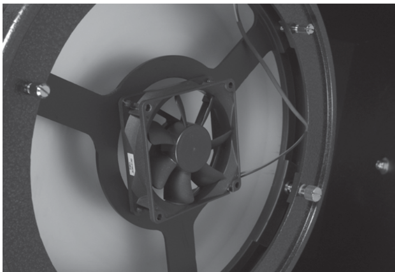
Figure 54-29 A mirror cooling fan is built into the base of the Zhumell Dobsonian telescope tube.
