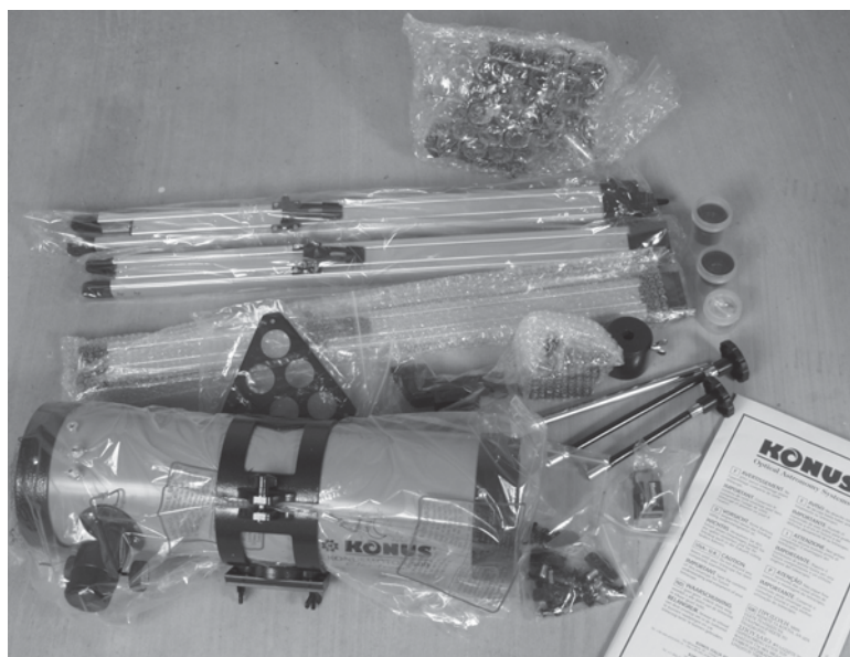
Figure 53-2 This is a highly portable, extremely powerful 4.5-inch Newtonian reflector telescope that accepts 1.25-inch eyepieces, uses a right ascension motor drive, and features a unique red laser dot “stardot” finder.
