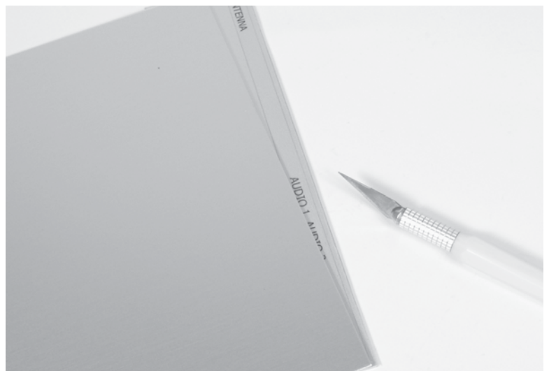
Figure 30-5 Trim the decal using the edge of the chassis bottom panel.
