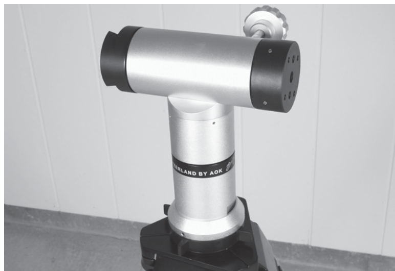
Figure 58-25 Carefully set the mount on top of the tripod mount plate.
