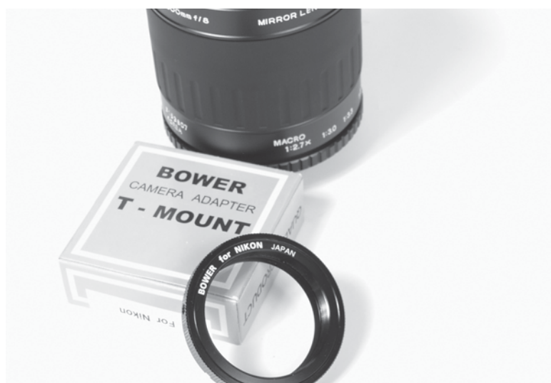
Figure 21-4 This mirror lens uses a “T-Mount” for attaching it to a camera. The interchangeable T-Mount (for example, just screw a different mount onto the lens; these mounts are available from a wide variety of different camera manufacturers) enables this lens to be used with different camera bodies.
