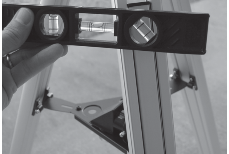
Figure 41-1 A small reliable spirit level is vital for establishing a useable telescope mount.
