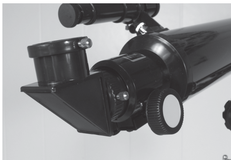
Figure 52-27 This diagonal can use 1.25-inch eyepieces.
