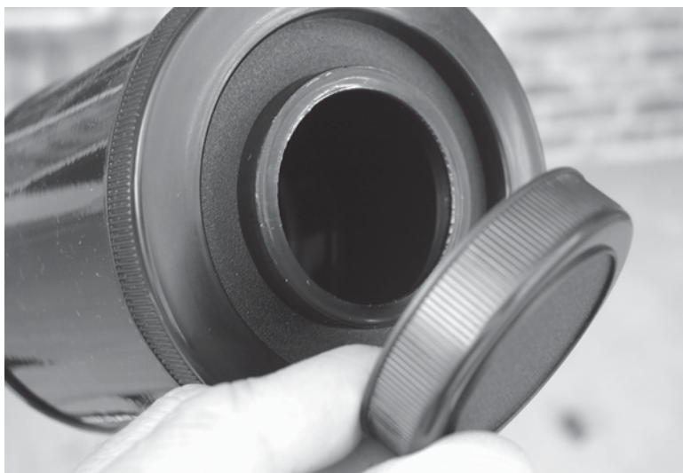
Figure 59-5 Remove only the center portion of your telescope's lens cap.
