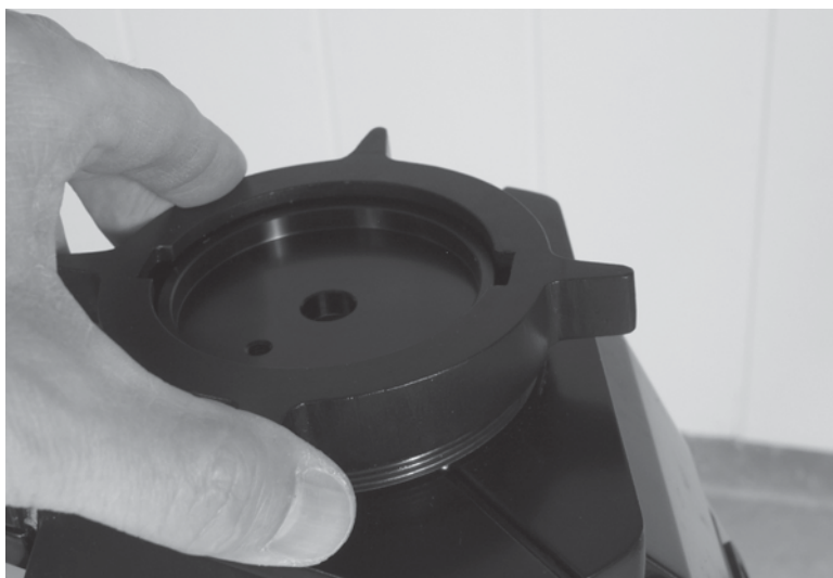
Figure 58-22 Reattach the tripod mount-locking nut.
