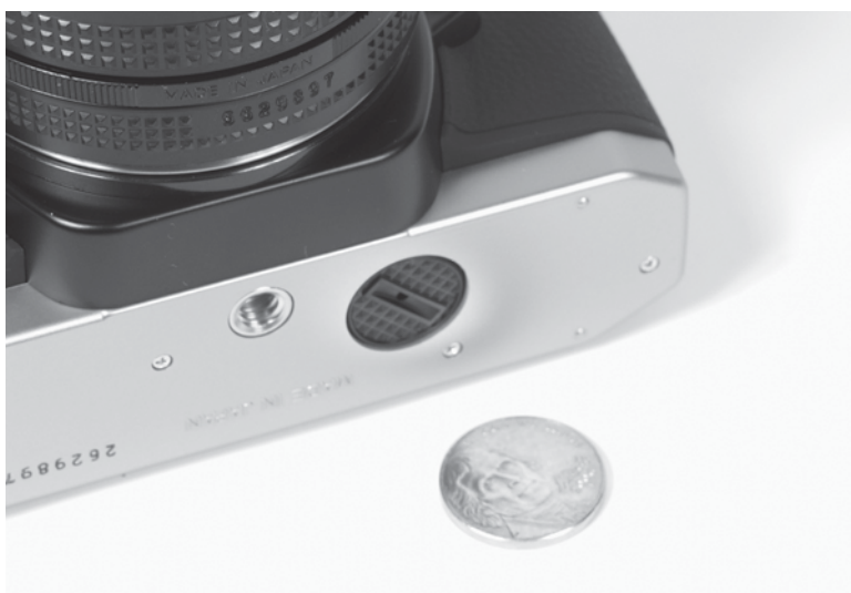
Figure 60-4 Only one little piece of modern technology is inside the FM10—a light meter battery. If you plan on using your film camera as a dedicated astrophotography camera, you won't need this newfangled contraption, so you can remove the battery.
