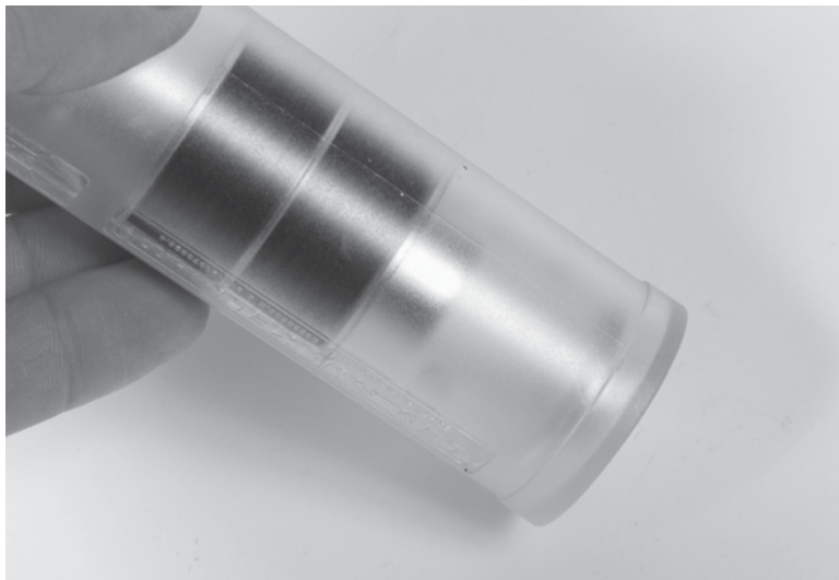
Figure 62-5 Power for the flashlight is provided by moving a magnet back and forth through a coil.
