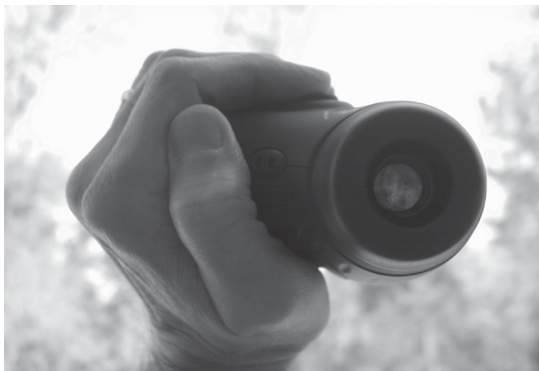
Figure 41-3 A Night Owl Optics Night Vision scope can be used for locating visual obstructions that might be blocking your telescope's field of view.
