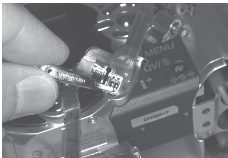
Figure 64-46 I dropped my lens assembly, but I retained the motors and switches that drive the lens, shutter, and aperture. To operate these switches, I have to short them with a clip during the camera startup sequence.
