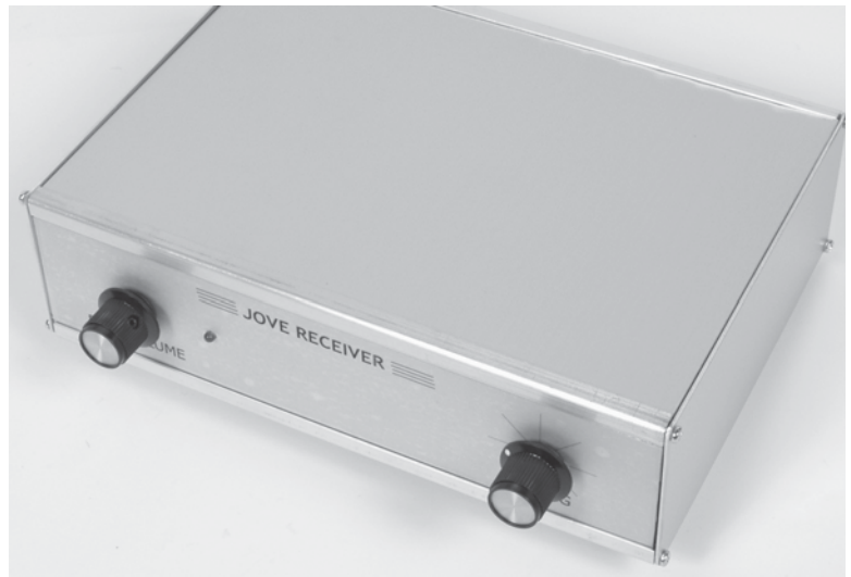
Figure 30-45 A Radio JOVE Receiver ready for listening to either Jupiter or the Sun.
