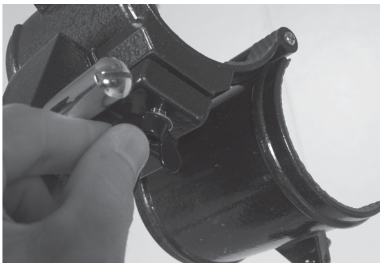
Figure 52-17 Attach the saddle to the telescope mount.
