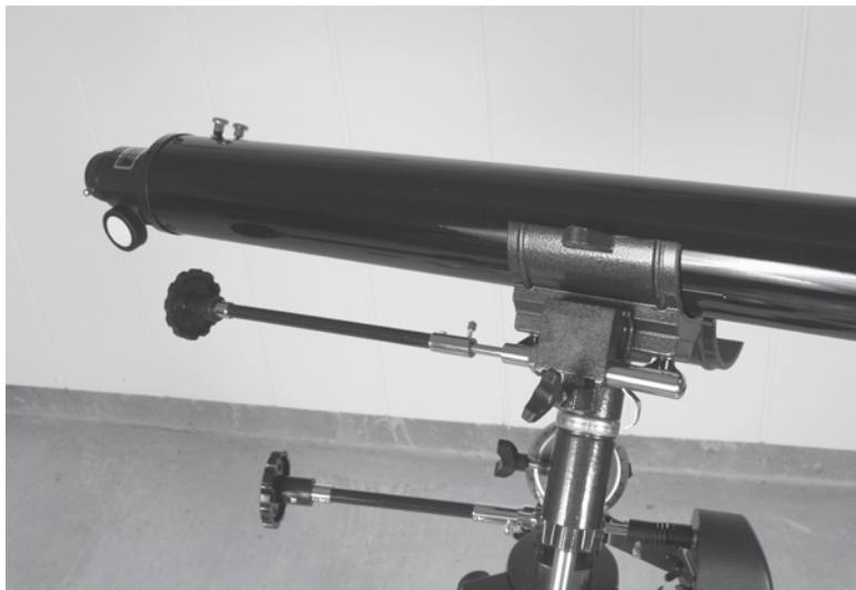
Figure 52-18 Gently lay the telescope tube in the saddle.
