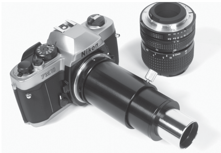
Figure 61-5 Mount the adapter on the camera and use the camera/adapter instead of an eyepiece.
