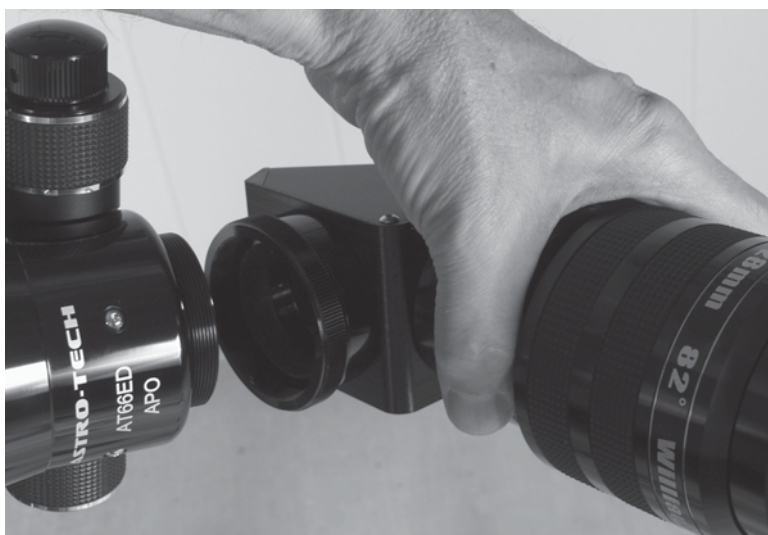
Figure 58-39 Mount the diagonal on the AT66ED refractor telescope.
