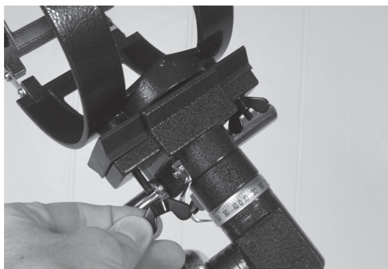
Figure 53-23 Attach the telescope saddle to the telescope mount.
