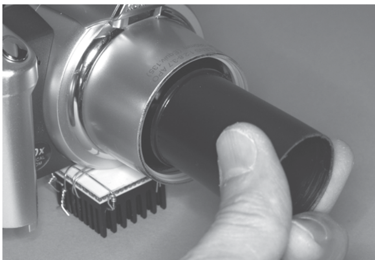
Figure 64-49 If you need one, a discarded 35mm film canister makes a great 1.25-inch eyepiece adapter.
