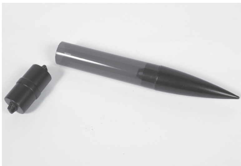
Figure 20-2 The nose cone connects to the payload tube without the typical recovery system attachment. Generally, the nose cone can be glued in place inside one end of the payload tube.
