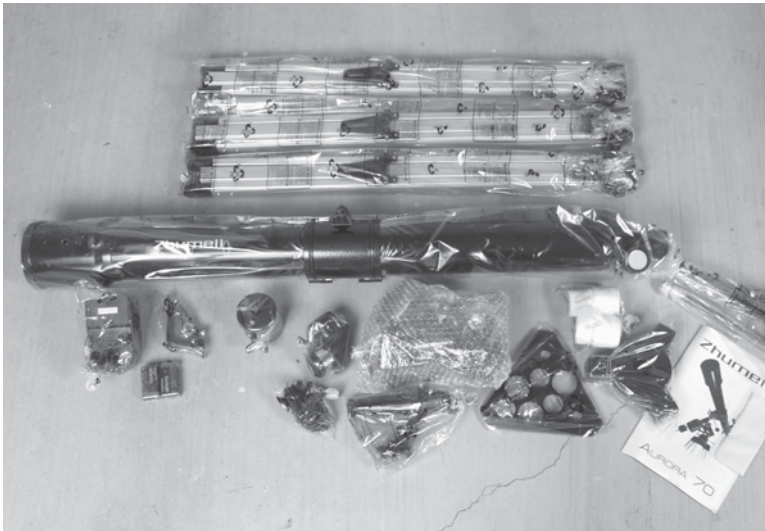
Figure 52-2 The Aurora 70 features a 70mm objective with a 900mm focal length, uses 1.25-inch eyepieces, and comes with a right ascension motor-drive mechanism.
