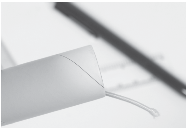
Figure 15–23 Pull the shock cord up and through the “other” end of the body tube.
