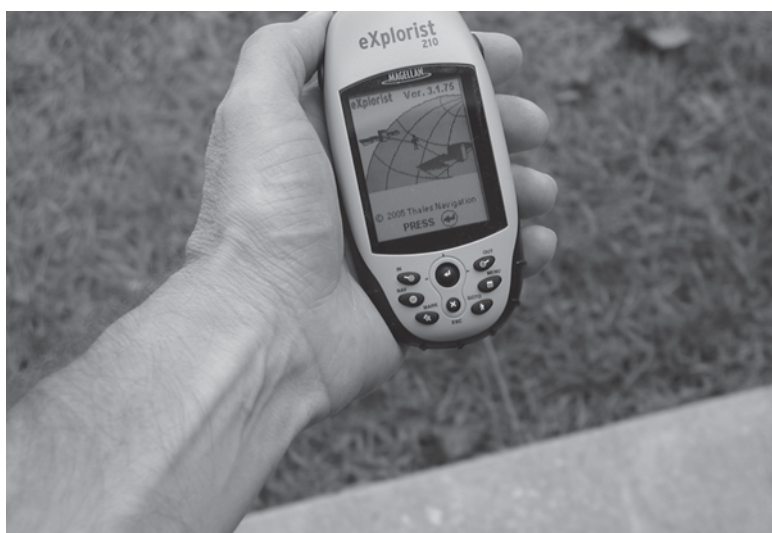
Figure 9-4 The first step is to help the GPS device find out where you are currently standing.
