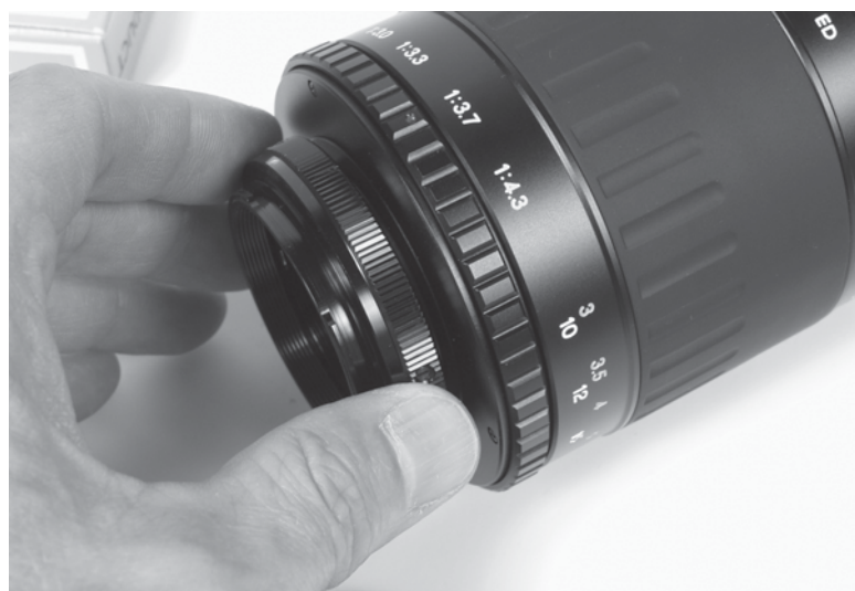
Figure 60-7 Find a T-Mount camera adapter. I removed one from this Vivitar 500mm mirror lens.
