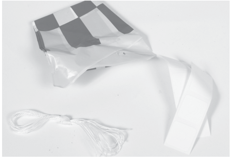
Figure 16-1 The materials needed for a parachute recovery system.
