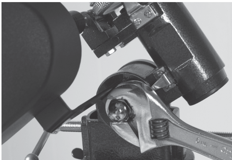
Figure 52-13 Reattach the nut from Figure 52-10 and securely fix the motor drive to the telescope mount.
