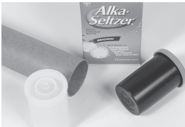
Figure 13-2 In addition to the antacid tablets, you also need an empty 35mm film canister. These two items are your motor mount and propellant. You also need a rocket body tube that can snugly and safely hold the motor mount (film canister).
