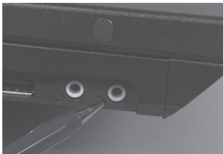
Figure 35-1 Beat those PC JOVE users at their own game. Make a Mac podcast of your Radio JOVE recordings. Use the Line In port of your computer to jack into the Radio JOVE Receiver.
