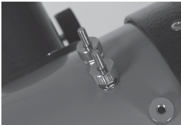
Figure 57-8 Most telescopes are predrilled for accepting a finder scope.
