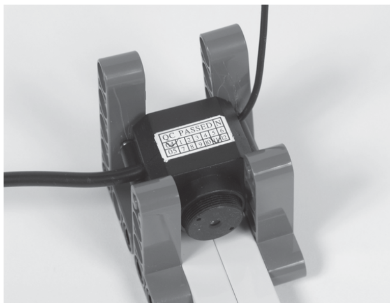
Figure 76-1 A miniature battery-powered video camera can be added to your robot for remote monitoring.
