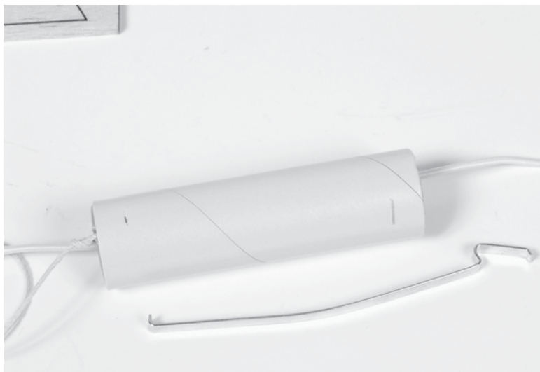
Figure 15-12 Slightly bend the motor retaining clip.
