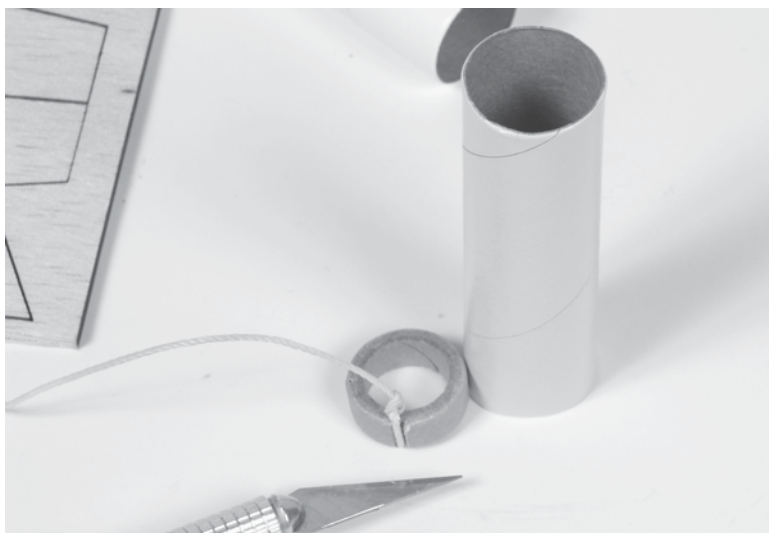
Figure 15-7 Measure the depth of the motor mount block on the motor mount.
