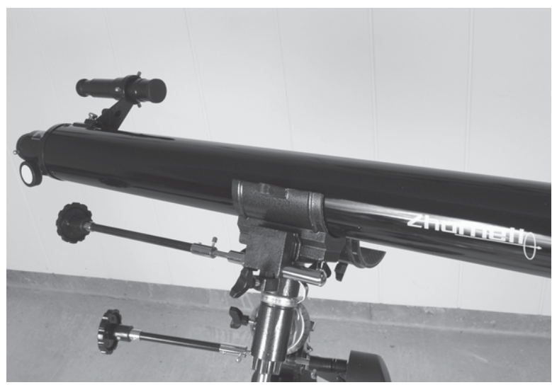
Figure 52-21 Attach the finder to the telescope tube, open the saddle again, and readjust the telescope's balance.
