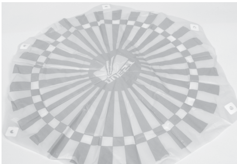
Figure 16-3 Spread the plastic out and attach all the reinforcement rings.
