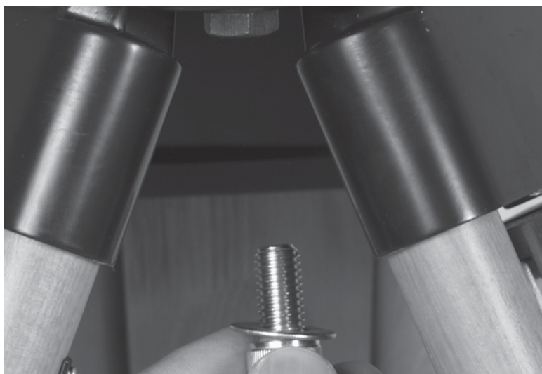
Figure 58-26 Insert the mount attachment bolt.
