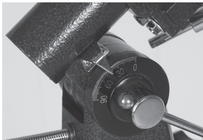
Figure 53-11 Elevate the telescope mount to approximately 45°.
