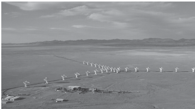
Figure 4-1 Aerial view of the Very Large Array (VLA), looking north-northeast; the antennas are in their closest configuration (D configuration). The National Radio Astronomy Observatory (NRAO) is a facility of the National Science Foundation, operated under cooperative agreement by Associated Universities, Inc. (AUI). (Photo by Dave Finley; Courtesy NRAO/AUI.)
