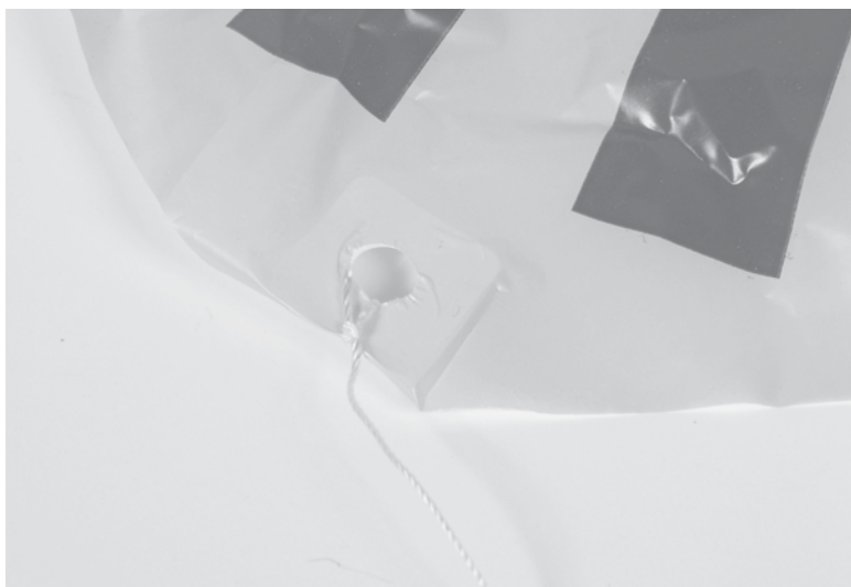
Figure 16-5 Tightly bind each end of the shroud line to the parachute.
