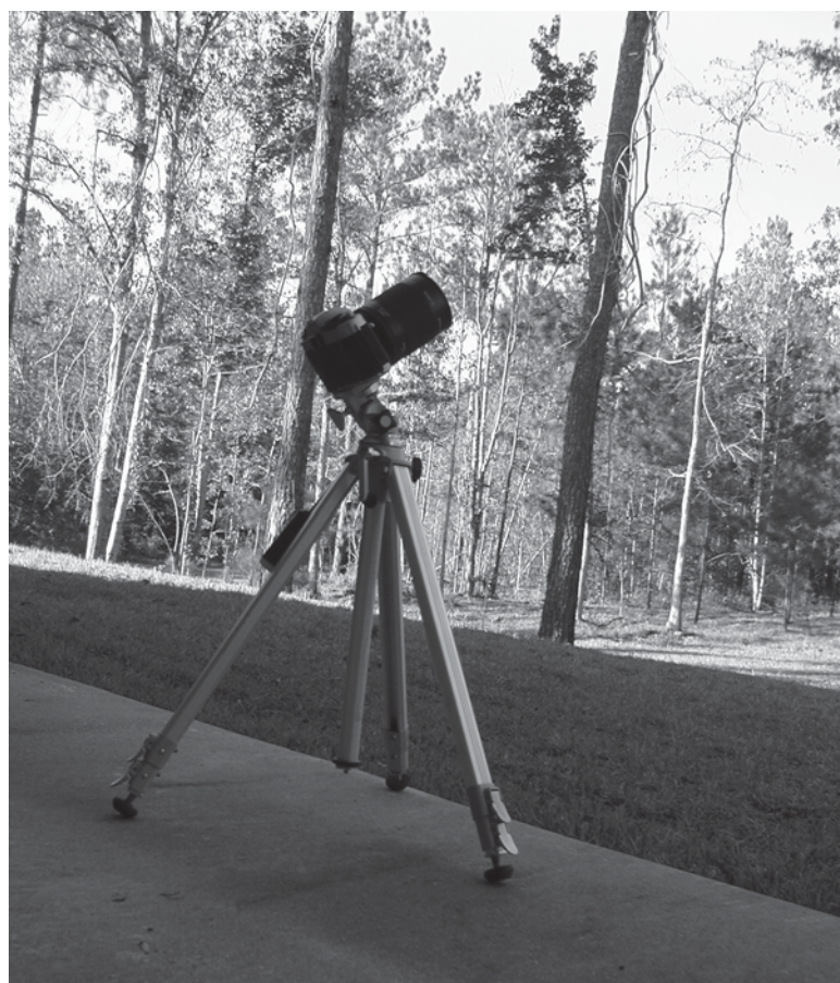
Figure 21-6 Attach the camera and mirror lens to a stable tripod for taking some deep-space photographs. This photograph was taken during the daylight hours.
