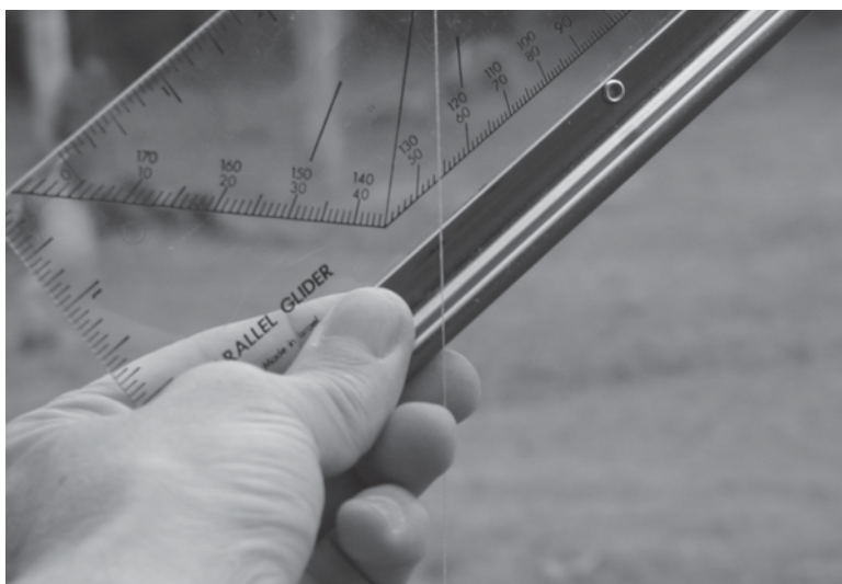
Figure 3-6 As you tilt the protractor, the thread indicates your viewing angle.
