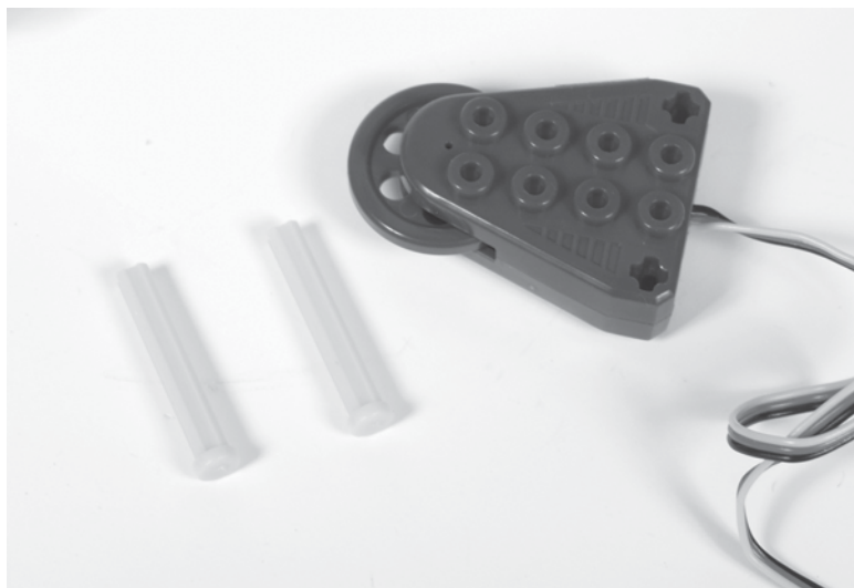
Figure 70-2 A touch sensor can be added to any design with just a couple of mounting pins.
