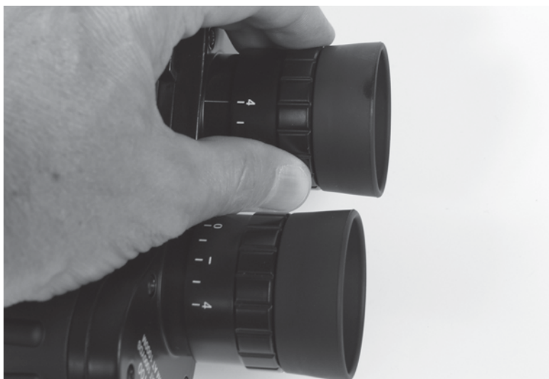
Figure 56-7 Unlike conventional binoculars, these astronomical binoculars are focused with the oculars. Each eyepiece must be individually focused.
