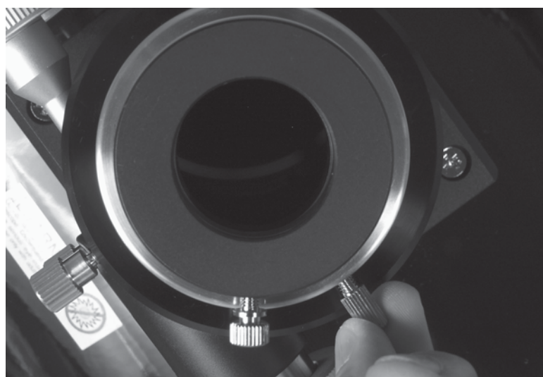
Figure 54-24 Remove the 1.25-inch eyepiece mount for installing a 2-inch eyepiece in the focuser.
