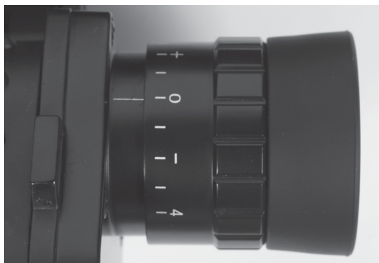
Figure 56-5 Each ocular is graduated for precision adjustment.
