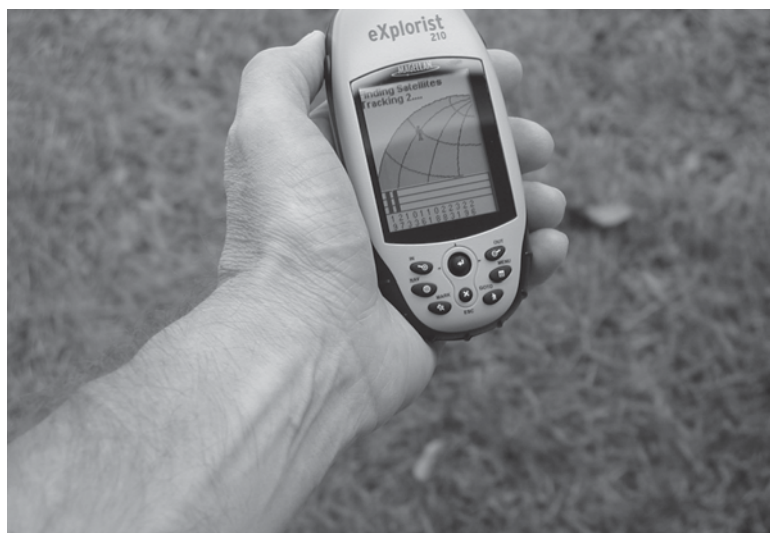
Figure 9-6 Two satellites have been located. Yes, you could now start using the GPS device, but for best results, you should wait until the eXplorist 210 indicates it has made a “3-D Fix” for your current position.
