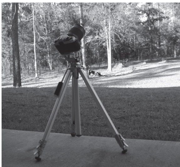
Figure 63-5 If you'd like to photograph star trails, then mount your camera on a conventional photography tripod and center your field-of-view on Polaris.
