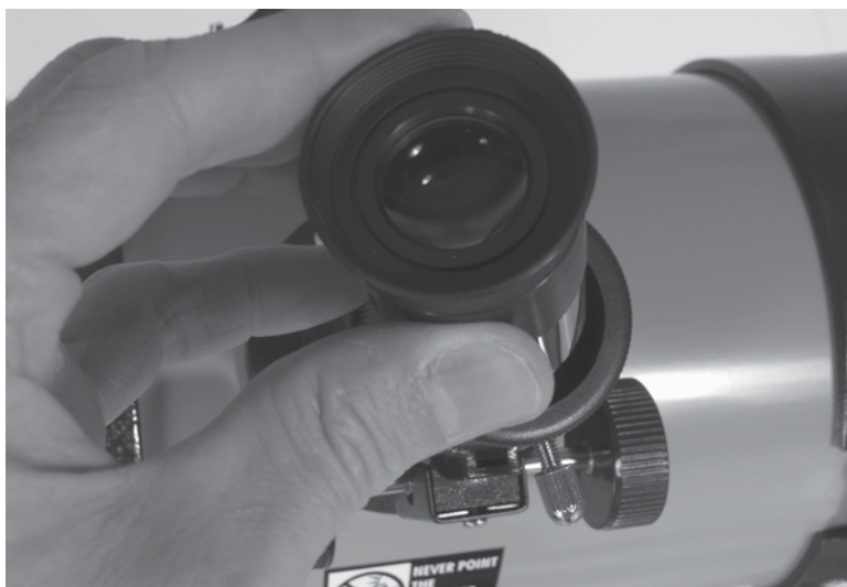
Figure 53-29 A set screw will hold the eyepiece in place.
