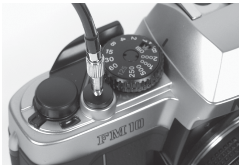
Figure 60-12 Ensure that you don't accidentally cross-thread the cable release.
