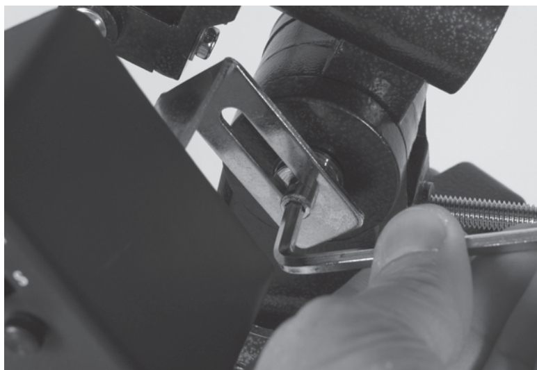
Figure 55-4 Attach the motor drive to the vertical adjustment bolt.
