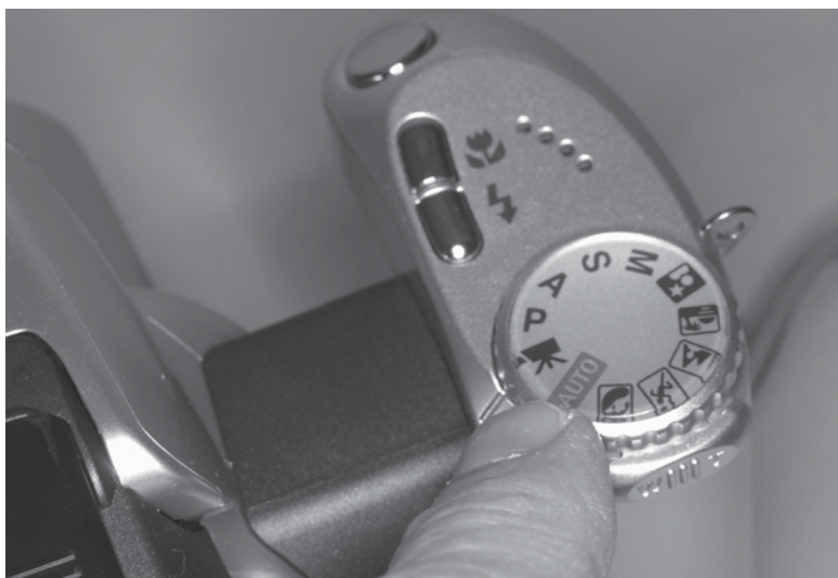
Figure 64-50 The video recording mode is more practical for using this CCD camera for astrophotography.
