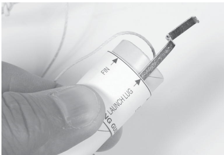
Figure 15-17 Line up the marking guide with the motor retaining clip, matching the mark for the launch lug.
