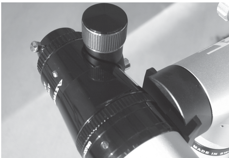
Figure 58-43 Either a diagonal or an eyepiece can be added to this telescope.
