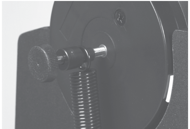
Figure 54-18 Gently set the telescope tube in the mount. Thread the spring mount into the pivot posts.
