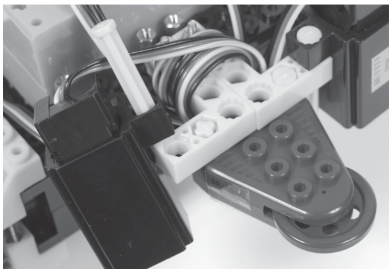
Figure 70-3 A touch sensor mounted alongside two light sensors.
