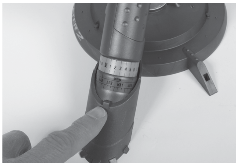
Figure 50-4 Turn the projection wand's dial until the desired month is lined up with the indicator mark.
