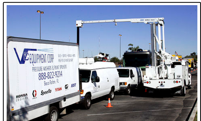
Security screening of cars at Super Bowl XLI using ^{60}\text{Co} gamma-ray scanner (2007)
