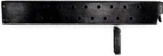
PHOTO 51: The magazine assembled and ready for the stop to be fitted.
