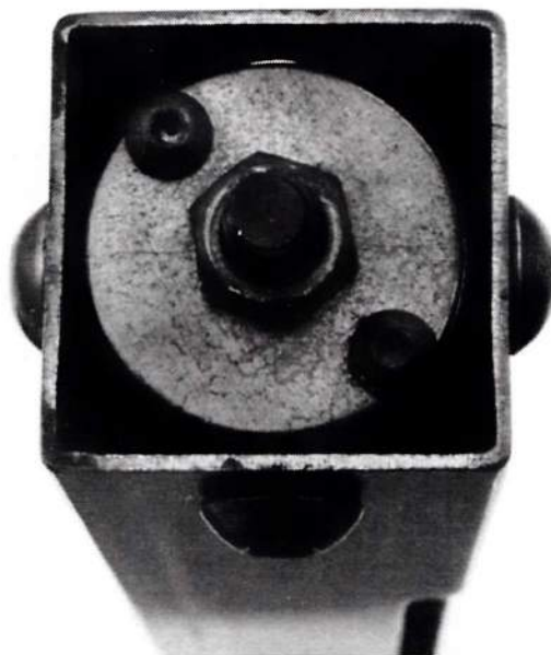
PHOTO 31: Rear view of upper receiver with recoil shield bolted in position.
