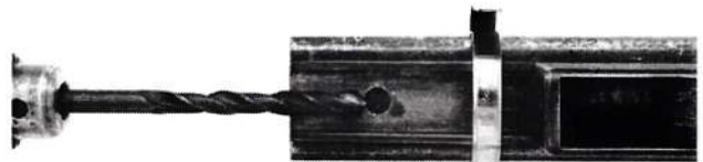
PHOTO 7: Drill through lower receiver bolt holes and into upper receiver tube.
