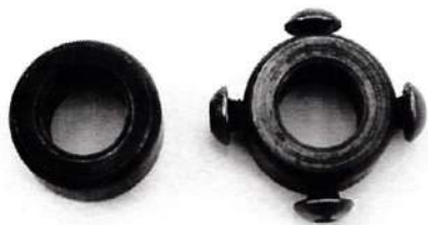
PHOTO 10: Steel collar shown alongside modified collar with four socket screws fitted.
