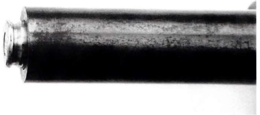
PHOTO 16: The base of the cartridge should protrude 4 mm from the breech face of the barrel.
