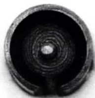
PHOTO 25: Firing pin fitted. The firing pin should not protrude more than 1.5 mm.
