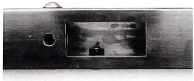
PHOTO 28: The ejector fitted to the receiver as seen through the magazine well recess.
