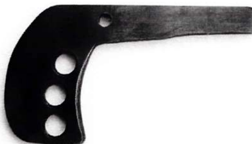
PHOTO 42: The trigger with all holes drilled.
