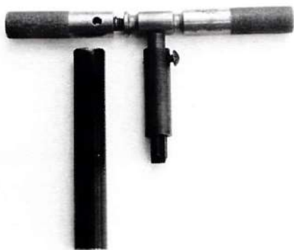
PHOTO 14: Complete reamer assembly. Sleeve is shown in position with reamer guide alongside.
