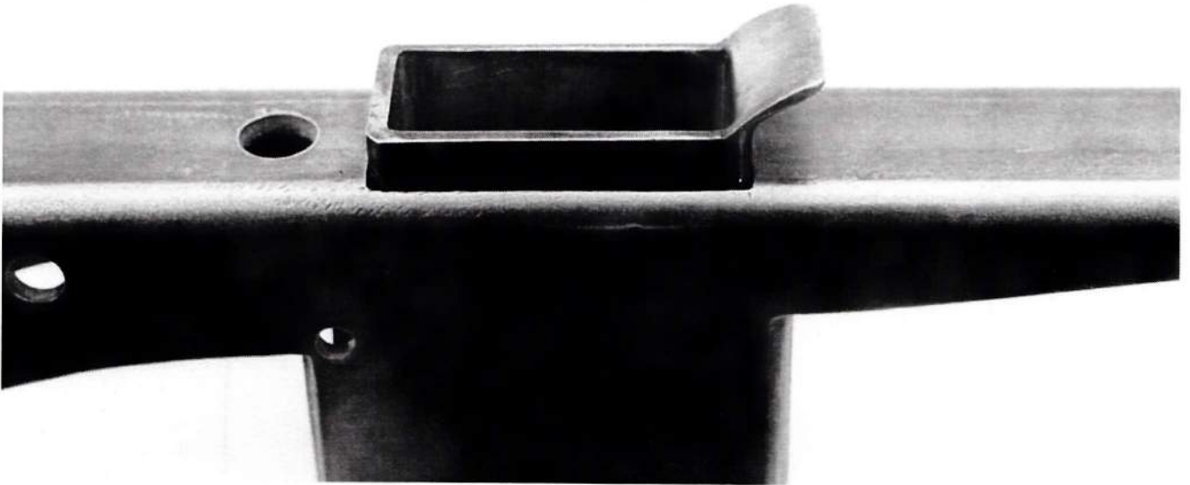
PHOTO 38: The magazine well, fitted in position.
