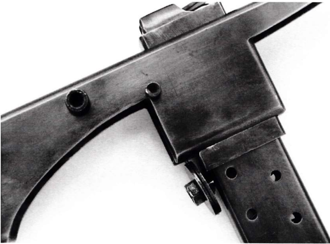
PHOTO 52: The magazine fitted. The magazine catch should hold the magazine firmly in position.
