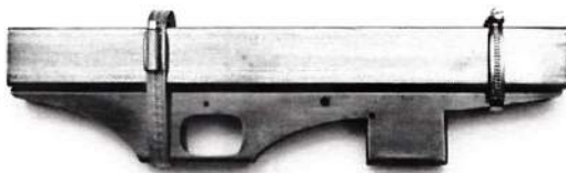
PHOTO 6: Upper and lower receivers clamped together with two hose clips.
