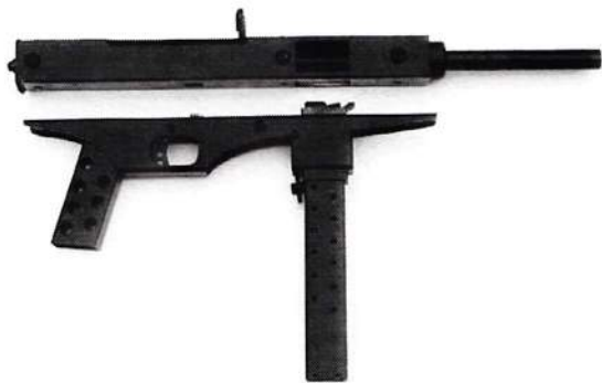
PHOTO 54: The two receivers ready to be bolted together.
