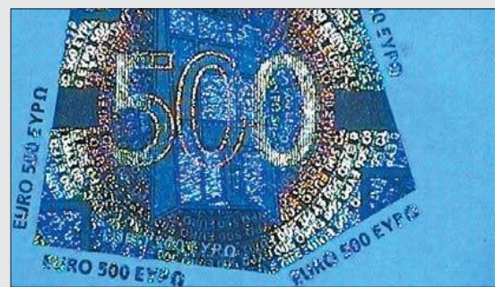
Below: OVDs revealed with LED illumination.
