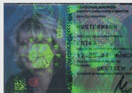
Below: OVDs revealed with LED illumination.
