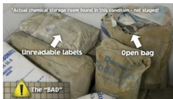
Figure 3. Example of improper chemical storage
