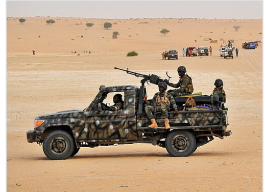
A Toyota Land Cruiser technical with a mounted Type 77 heavy machine gun in N'Gourti, Niger , 2019
