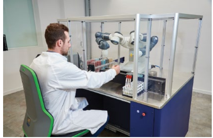
Figure 40-10 Additional modules. Shown here are components of the WASPLab, including the WASP-FLO (A) and Collaborative Robot (B). The WASP-FLO module can be used for streamlining samples in laboratories in which multiple sample processors are being used. It automatically sorts samples and directs them to the appropriate WASP DT. The Collaborative Robot module assists with manual processing of positive blood cultures, tissues, and traditional swabs. (Photo courtesy of Copan Diagnostics, Murrieta, CA.)
