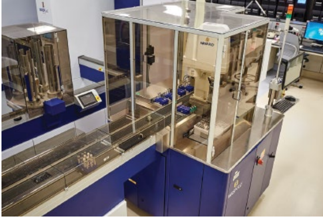
Figure 40-10 Additional modules. Shown here are components of the WASPLab, including the WASP-FLO (A) and Collaborative Robot (B). The WASP-FLO module can be used for streamlining samples in laboratories in which multiple sample processors are being used. It automatically sorts samples and directs them to the appropriate WASP DT. The Collaborative Robot module assists with manual processing of positive blood cultures, tissues, and traditional swabs. (Photo courtesy of Copan Diagnostics, Murrieta, CA.)
