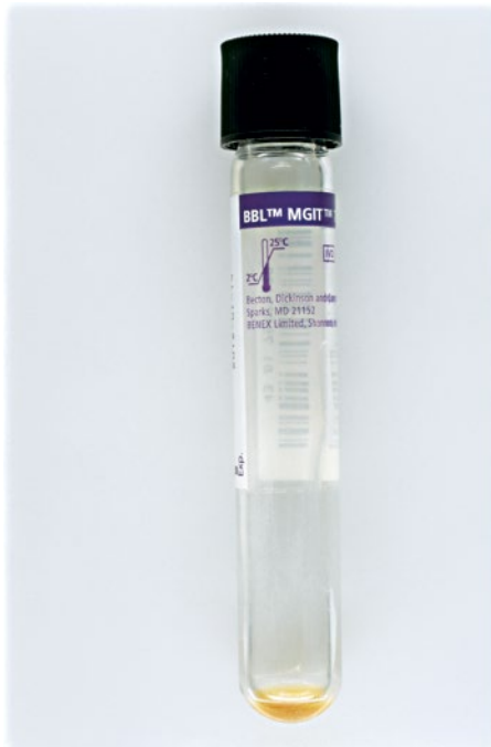
Figure 9-31 BD BACTEC MGIT. BD BACTEC MGIT (mycobacterial growth indicator tubes) (BD Diagnostic Systems, Franklin Lakes, NJ) use fluorometric technology to expedite the reading of results. Positive tests emit an orange fluorescent glow at the base of the tube and at the meniscus that can be read using a Wood's lamp or other long-wave UV light source, or they can be incubated and read in the BD BACTEC 960 Instrumented Mycobacterial Growth System.
